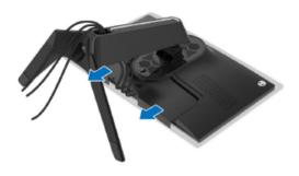
Disconnect the cables from the monitor and slide them out through the cable-management slot on the stand riser.
