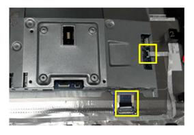
S16 Unlock 15 screws to disassemble Middle Frame from Panel
