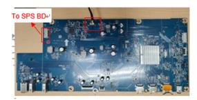
S29 Disassemble SPS BD from Main SHD and disassemble "AC Socket Wire" from SPS BD
