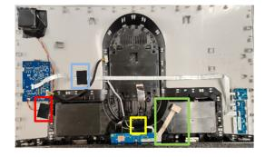
S10 Unlock 2 USB screws to disassemble USB BD from Rear Cover
