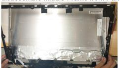
S18 Tear off a tape on backlight wire and unplug backlight wire from panel
