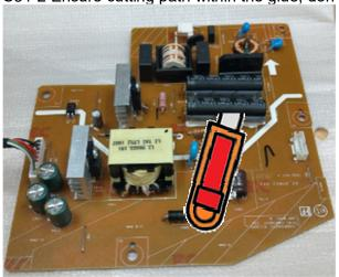
S31-3 Take out bulk cap. pin solder with soldering iron and absorber
