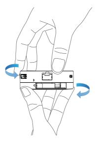
2. With the USB-C cable facing you, turn the top section to release the USB-C cable.
