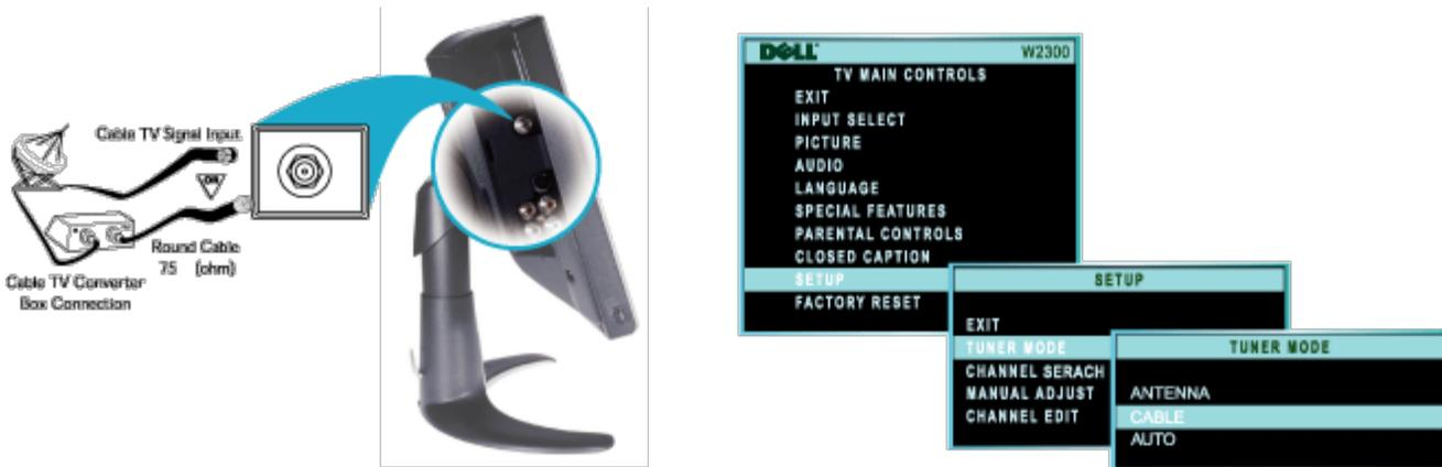
1. If your Cable TV signal is a single, round cable (75 ohm), then you're ready to connect to the TV. Connect the TV cable to the ANTENNA/CABLE plug on the TV.
