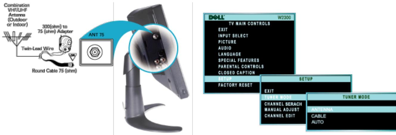
1. If your antenna has a round cable (75 ohm) on the end, then you're ready to connect it to the TV. If your antenna has flat, twin-lead wire (300 ohm), you first need to attach the antenna wires to the screws on a 300 -to 75- ohm adapter.
