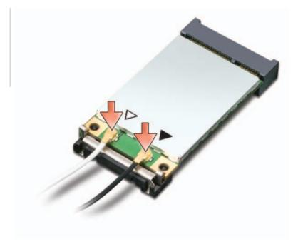
Connect the appropriate antenna cables to the Mobile Broadband card you are installing. To do so, connect the white with gray striped cable to the connector on the card marked by a white triangle. Connect the black with gray striped cable to the connector on the card marked by a black triangle.
