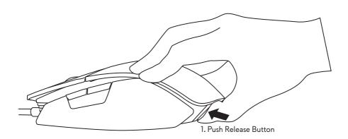
**2.** While holding down the release button, slide the palm rest backwards either 1 notch or 2 notches to suit your palm size.
