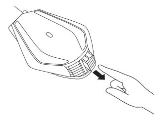
**2.** Each 5 gram weight (4 pieces in total) can be removed by sliding it out from the carrier casing
