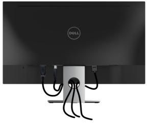
After attaching all necessary cables to your monitor and computer, (see Connecting Your Monitor for cable attachment) organize all cables as shown above.
