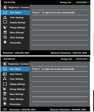
The following dialog appears on a black screen as the monitor self-adjusts to the current input:
