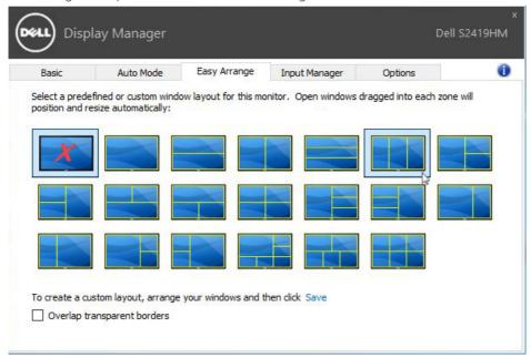
To create a custom window layout, size and position the windows (maximum 10) on the desktop and then click the **Save** link in **Easy Arrange**. The size and position of the windows is saved as a custom layout and the custom layout icon is created.
