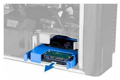
**6.** If a 2.5-inch hard drive is installed, remove the screws and lift up the drive to remove it from the hard-drive caddy.
