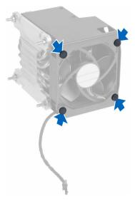
**4.** Slide the heatsink fan from the heatsink assembly.
