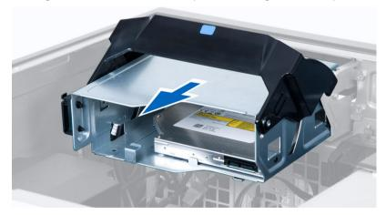
**9.** Remove the screws that secure the optical drive to the optical-drive cage.
