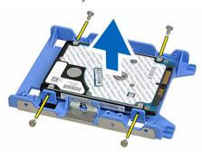
7. If a 3.5-inch hard drive is installed, flex the hard-drive bracket on both sides to loosen the hard drive.
