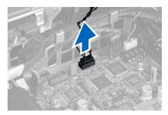
5. Release the latch that secures the HDD thermal sensor. Here, the HDD thermal sensor is attached to the hard drive.
