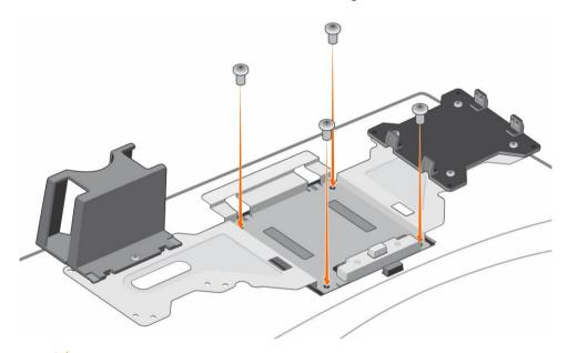
CAUTION: If you need to remove the P-series mount, remove the monitor screws and then press the lower quick release button(in black) on the monitor, not the upper release button(in silver) on the mount.
