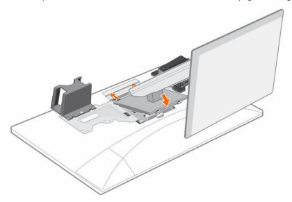
5 Attaching the client— Place the client over the bracket and gently push the client untill it clicks.
