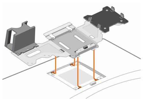
—Install the P-series mount to the back of the monitor using the four monitor screws set aside earlier (do not over-tighten).
