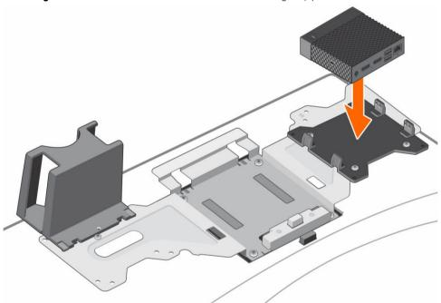
(i) NOTE: The power button of the client must face upward.
