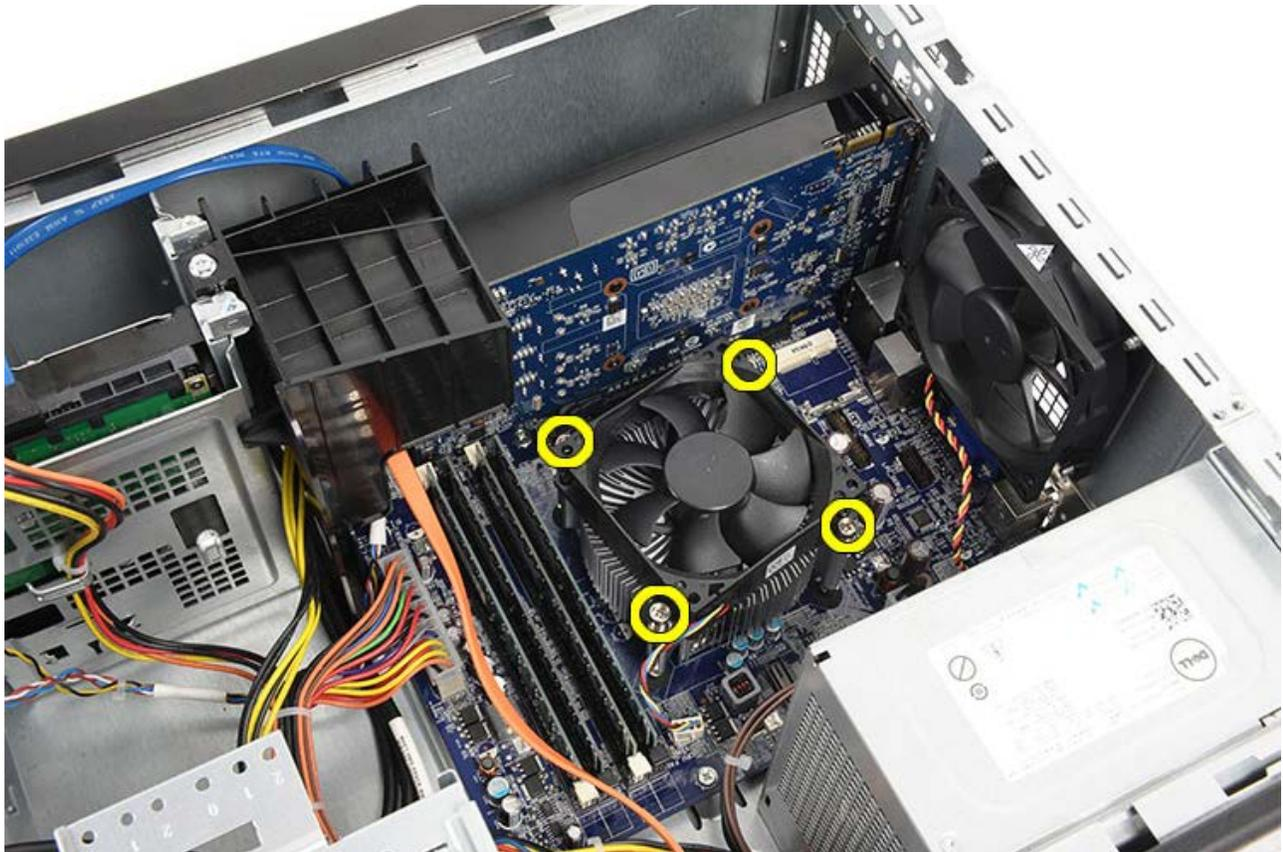
5. Lift the heat sink/fan assembly upward gently, and remove it from the computer. Lay the assembly with the fan facing downward, and with the thermal grease facing upward.
