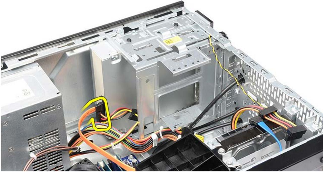
5. Remove the screws that secure the optical drive to the drive cage.
