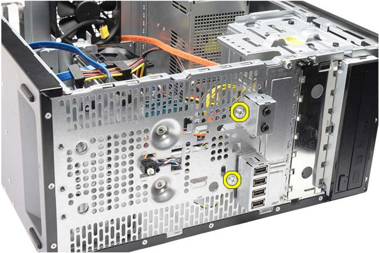
8. Ease the front I/O panel away from the computer as you guide the cables through the bays and holes.
