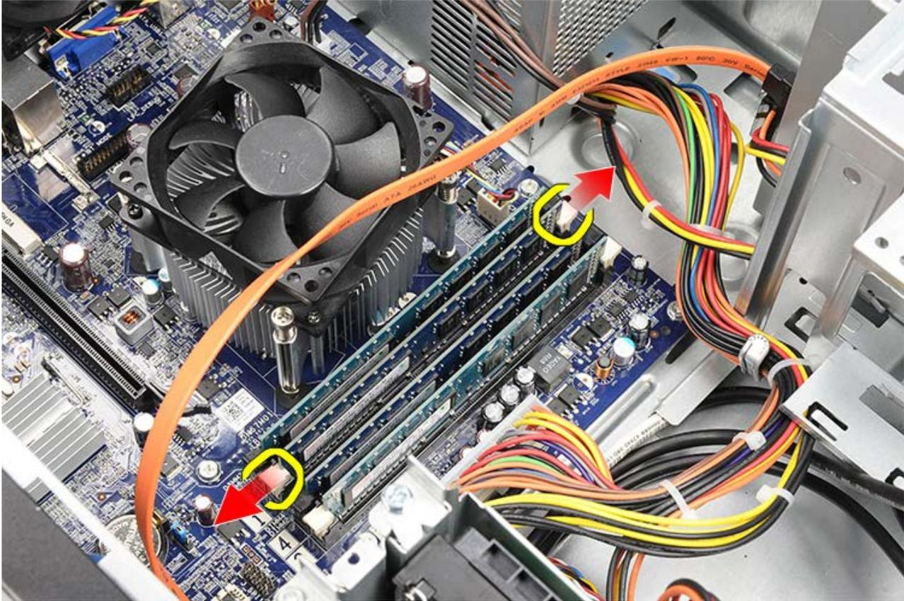
5. Grasp the memory module and pull it out of the memory module connector.
