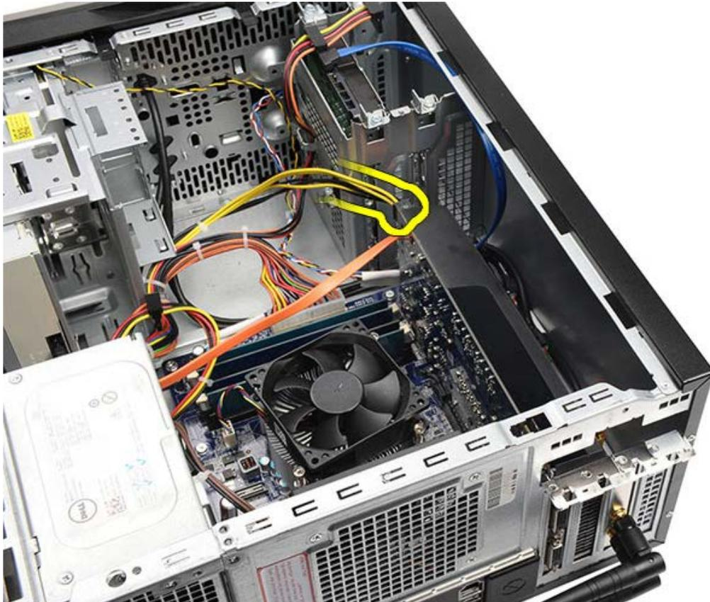
7. If a PCI-express x16 video card is installed, press the securing tab.
