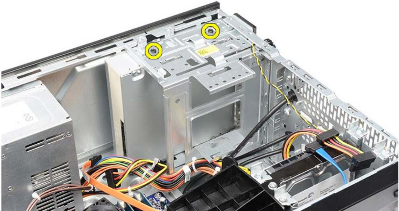
6. Slide out the optical drive through the front of the computer.
