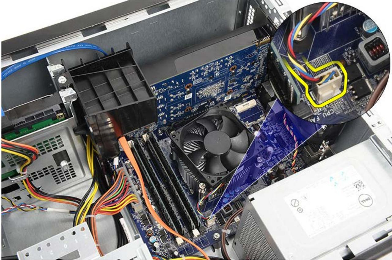
4. Loosen the four captive screws that secure the heat sink/fan assembly to the system board.
