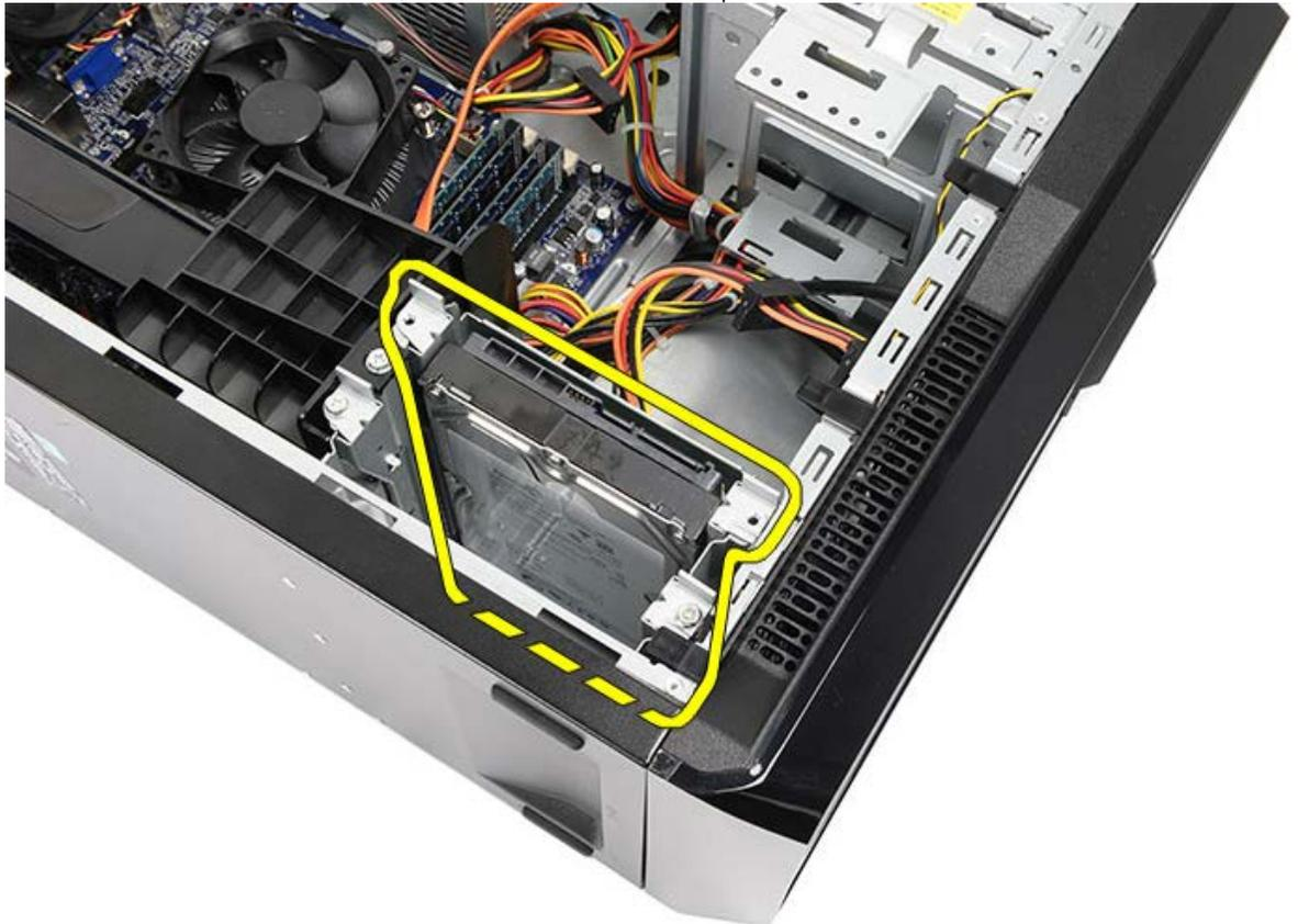
6. Remove the two screws securing the hard drive to the drive cage.
