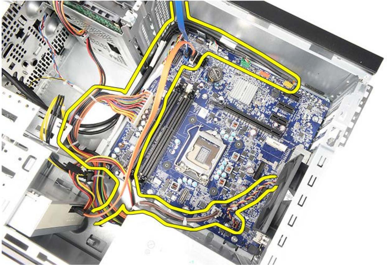
10. Remove the eight screws that secure the system board to the computer.
