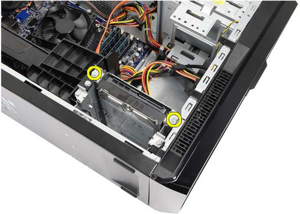
5. Slide the hard drive out of the slot, toward the side of the computer.
