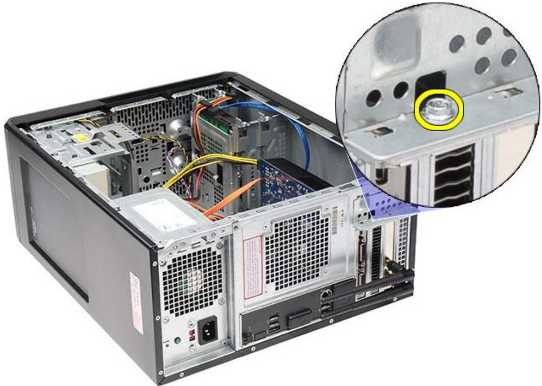
5. Remove the metal securing tab away from the computer.
