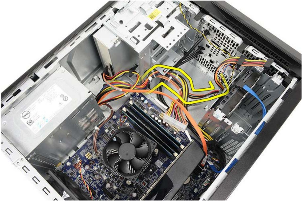
6. Remove the screws that secure the power supply to the computer chassis.
