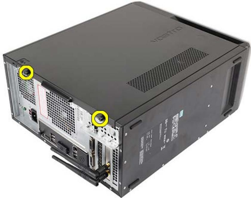
3. Slide the computer cover towards the back of the computer, and then remove it from the computer.
