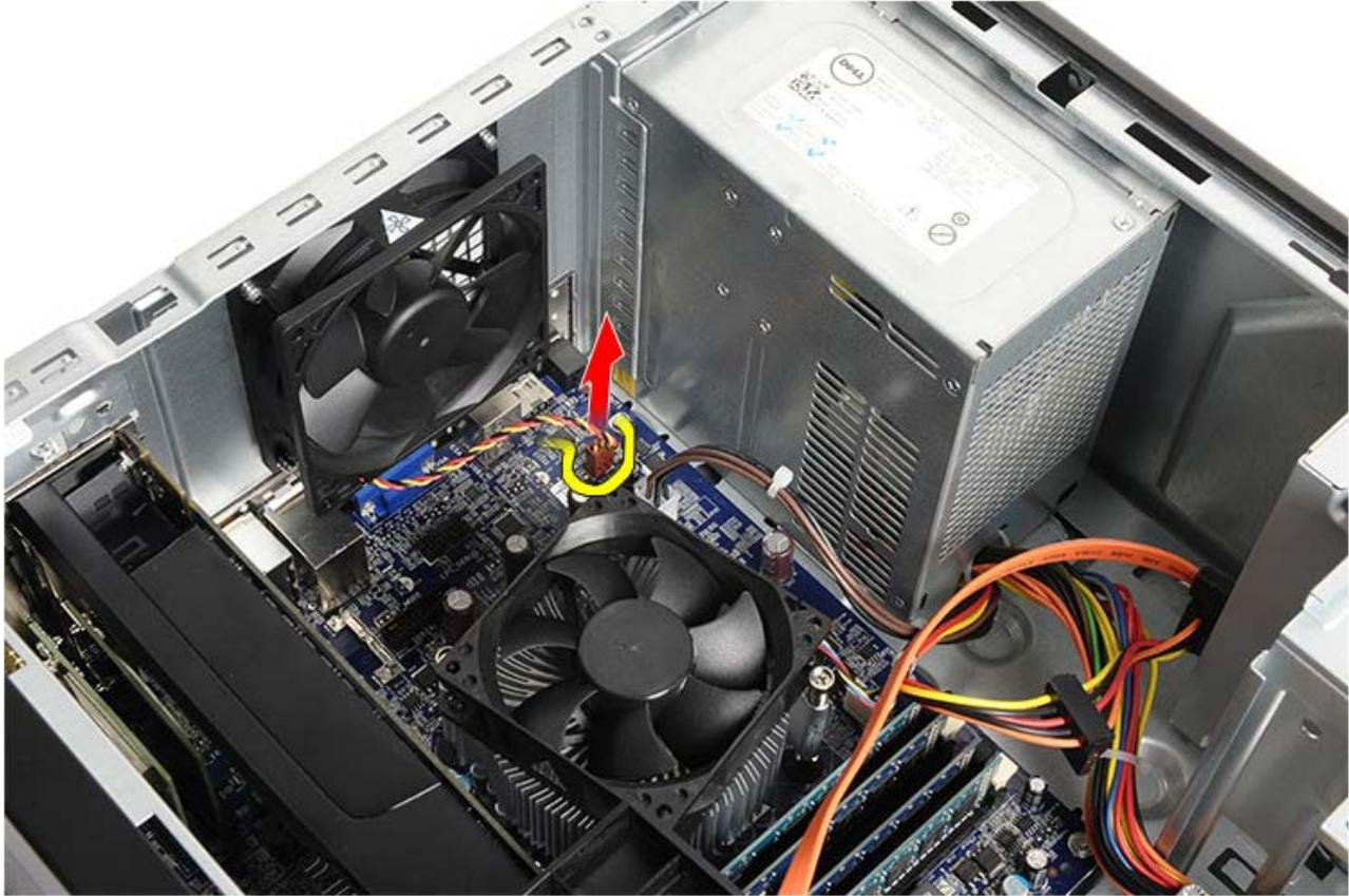
4. While holding the chassis fan in place, remove the four screws that secure the fan to the chassis.
