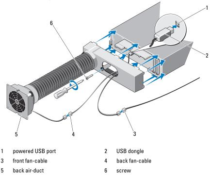
**9** Replace the screw to secure the back air-duct to the computer.
