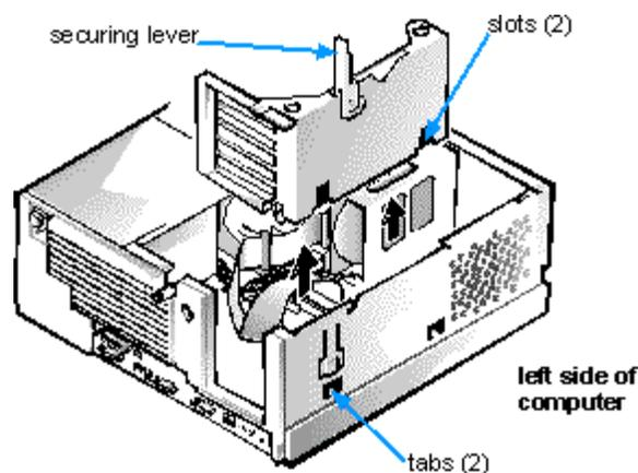
4. Slide the expansion-card cage out of the chassis.
