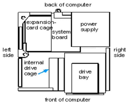
[Figure 5](#) shows your computer with its cover removed. Refer to this illustration to locate interior features and components discussed in this guide.
