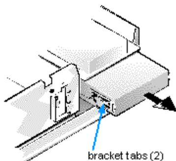
If a drive is already installed in the bay and you are replacing it, be sure to disconnect the DC power cable and interface cable from the back of the drive before sliding the bracket out of the bay. To remove the old drive from the bracket, turn the drive/bracket assembly upside down and unscrew the
