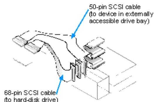
**NOTICE: Do not connect devices to all three connectors (internal narrow connector, internal wide connector, and external connector) on a single SCSI host adapter card. Such a configuration is a violation of the SCSI specification. You can safely connect devices to any two of these three connectors on a single SCSI host adapter card.**
