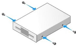
4. Align the shoulder screws on the floppy drive with the shoulder screw slots, and gently slide it into the bay until it clicks into place.
