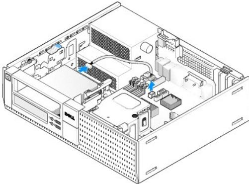
4. Lift the drive-release latch and slide the media card reader toward the back of the computer. Then, lift it out of the chassis.
