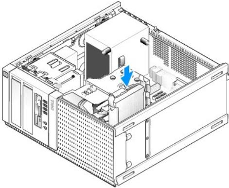
8. Connect the power and data cables to the drive(s).
