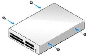
4. Align the shoulder screws with the screw guides in the mounting rack, and slide the media card reader into the bay until it clicks into place.
