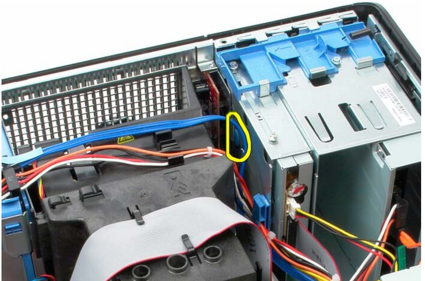
6. Vip IO-panelet imod systemets bagside.
