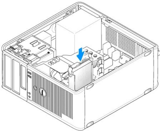
8. Attach the SATA data cable removed in [step 5](#) to the first hard drive.
