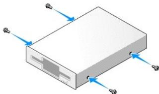
6. Align the shoulder screws on the floppy drive with the shoulder screw slots, and gently slide the drive into the bay until it clicks into place.
