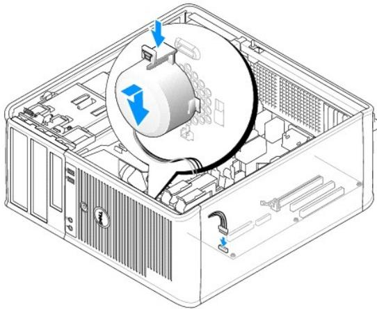
4. Connect the cables to the system board.
