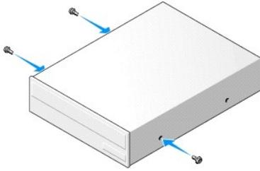
5. Align the shoulder screws on the optical drive with the shoulder screw slots, and slide the drive into the bay until it clicks into place.
