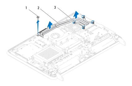
1 screw 2 processor heat-sink
