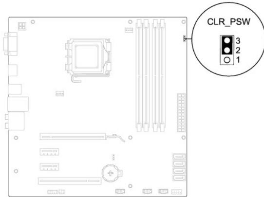
4. Remove the 2-pin jumper plug from pins 2 and 3 and fix it on pins 1 and 2.
