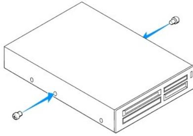
4. Gently slide the Media Card Reader into place in the FlexBay slot, until the Media Card Reader snaps into place.
