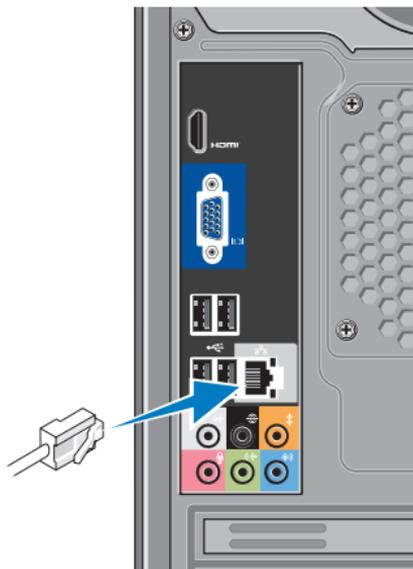
A network connection is not required to complete your computer setup, but if you have an existing network or Internet connection that uses a cable connection (such as a home cable modem or Ethernet jack), you can connect it now. Use only an Ethernet cable (RJ45 connector). Do not plug a telephone cable (RJ11 connector) into the network connector.
