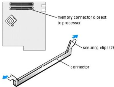
5. Align the notch on the bottom of the module with the crossbar in the connector.
