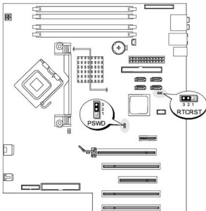
2. Locate the 3-pin password jumper (PSWD) on the system board, and remove the jumper plug from pins 1 and 2.
