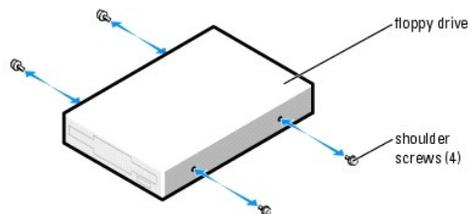
2. Slide the floppy drive into the floppy drive bay until the sliding plate clicks into place and the drive snaps into position.
