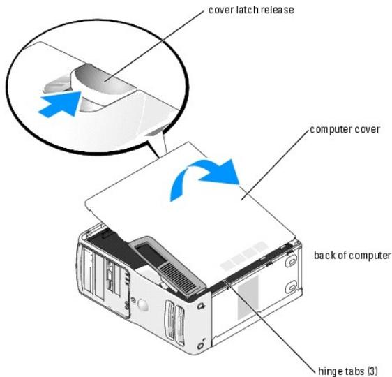
5. Locate the three hinge tabs on the bottom edge of the computer.
