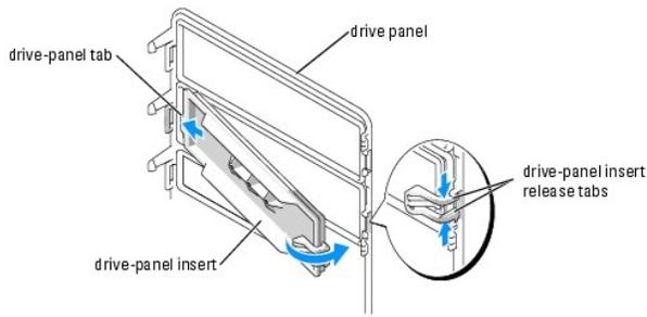
3. Ensure that the drive-panel insert is correctly seated in the drive panel.
