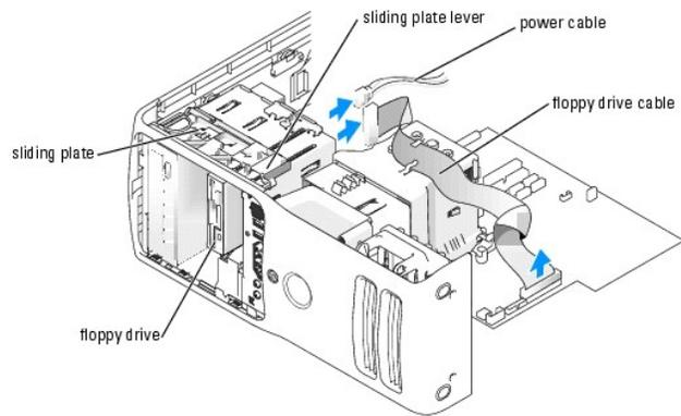
5. Pull the sliding plate to the right and hold in place.
