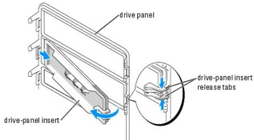
**NOTE:** To avoid breaking the drive-panel insert tab, do not pull the insert more than approximately 1 cm (1/2 inch) away from the drive panel before sliding the tab out of the slot.
