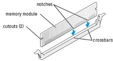
➡ **NOTICE:** To avoid damage to the memory module, press the module straight down into the connector while you apply equal force to each end of the module.
