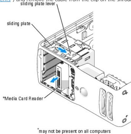
6. While pushing on the back of the drive, remove the Media Card Reader by sliding and holding the sliding plate.
