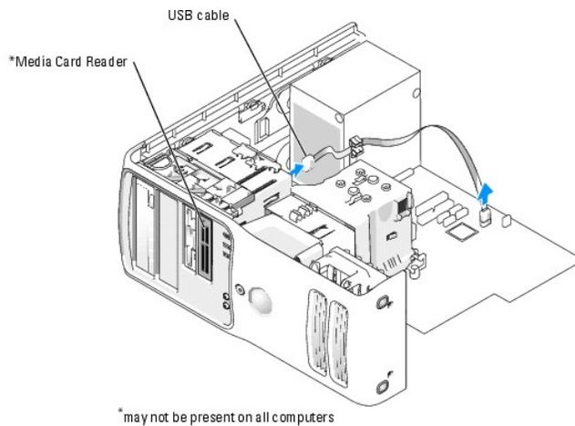
5. Disconnect the USB cable on the back of the Media Card Reader from the front panel USB connector on the system board (see "[System Board Components](#)") and remove the cable from the clip on the shroud.
