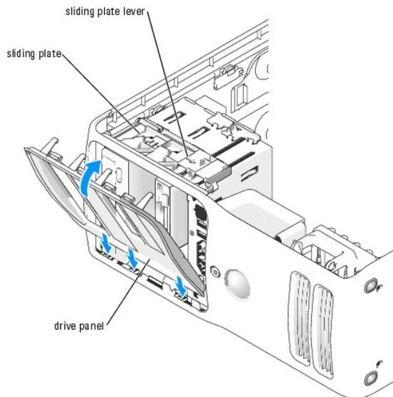
2. Align the drive panel tabs with the side-door hinges.
