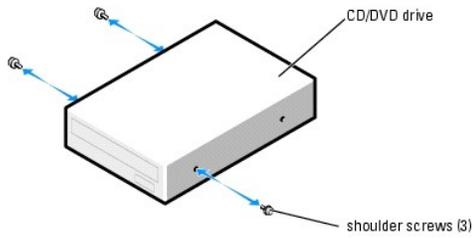
3. Slide the drive into the drive bay until the drive clicks into position.
