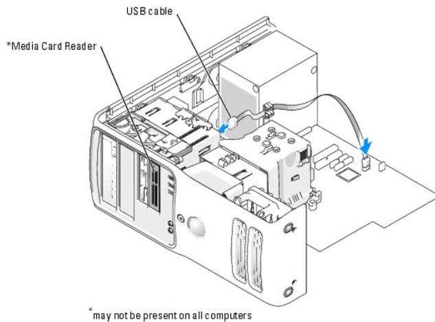
8. Insert the Media Card Reader into the bay and slide the drive in to seat it in the computer.
