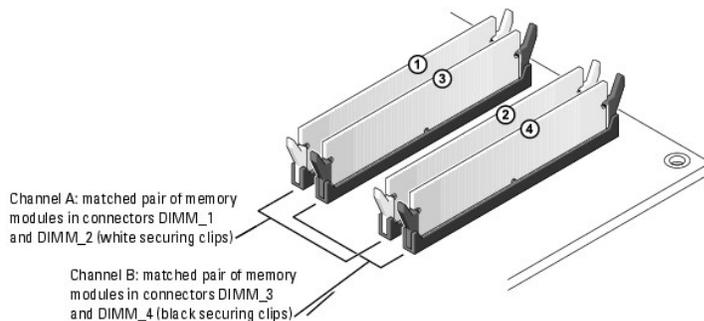
Channel A: matched pair of memory modules in connectors DIMM\_1 and DIMM\_2 (white securing clips)
