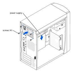
9. Remove the power supply from the computer.
