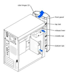
To reattach the front panel, attach the side hinges and then rotate the front panel until it snaps onto the front of the computer.
