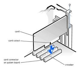
Ensure that the card is fully seated and that its bracket is within the card slot.
