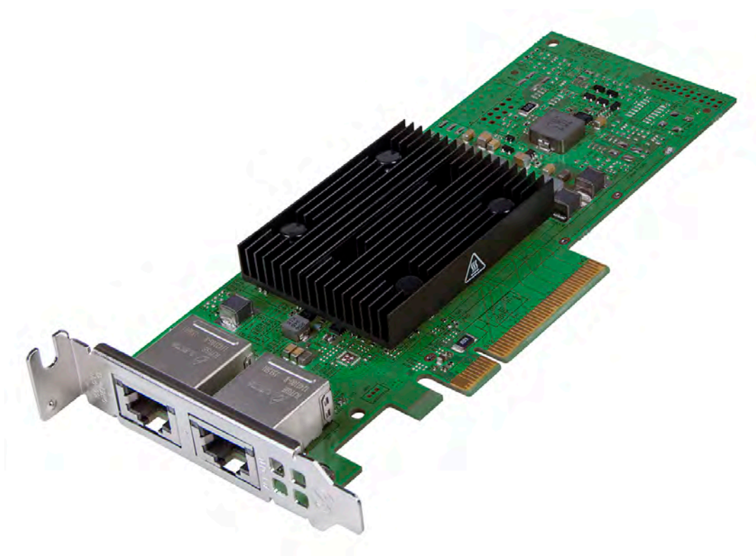
Figure 3: BCM957416A4160D Network Interface Card
