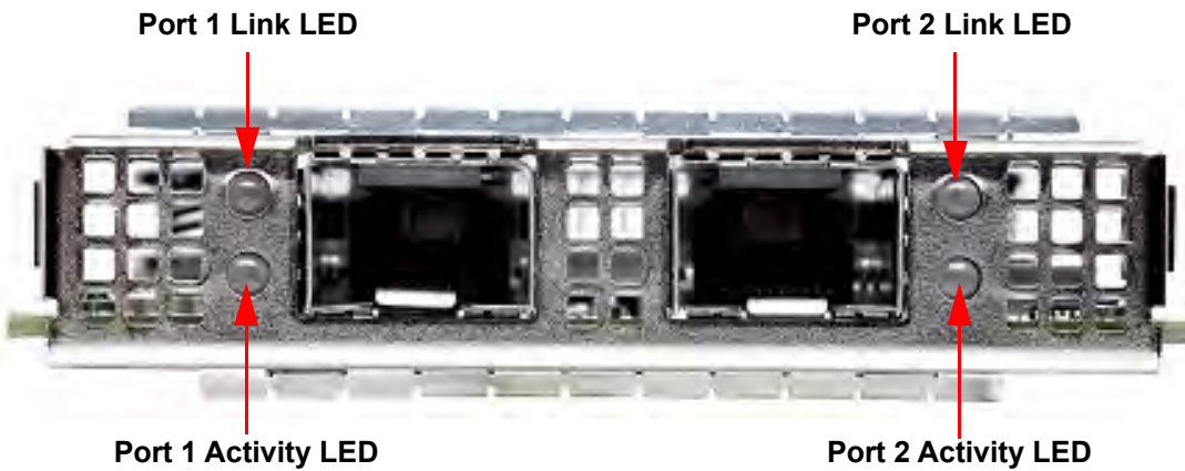
Figure 24: BCM957412N4120DC Network Adapter Activity and Link LED Locations
