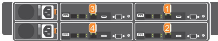
Figure 4. Enumeration four system boards for 1U node
