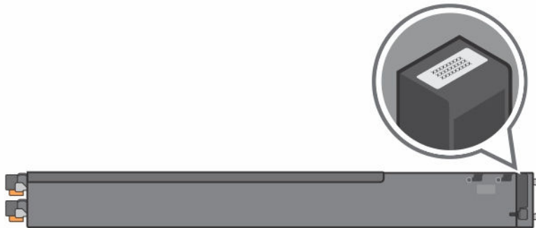
Figure 39. Service Tag location on the left front panel
