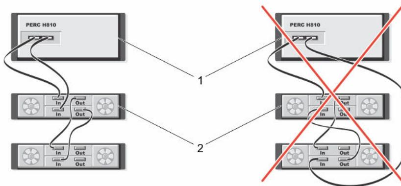
**Figure 4. Redundant Path Support Configuration With Two Enclosures**
