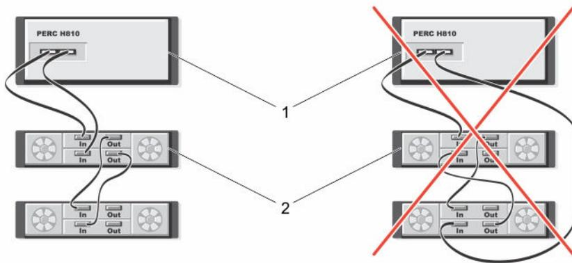
**Figure 4. Redundant Path Support Configuration With Two Enclosures**
