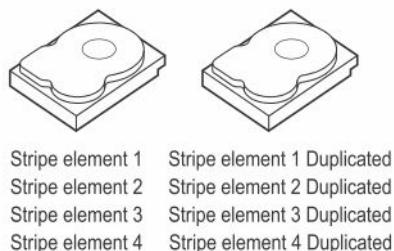
**Figure 7. Example of Disk Mirroring (RAID 1)**
