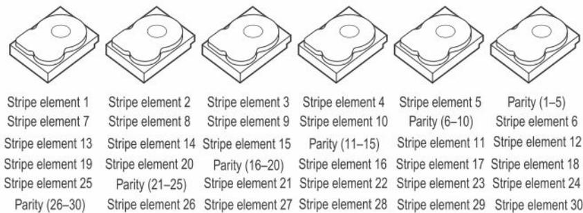
**Figure 8. Example of Distributed Parity (RAID 5)**
