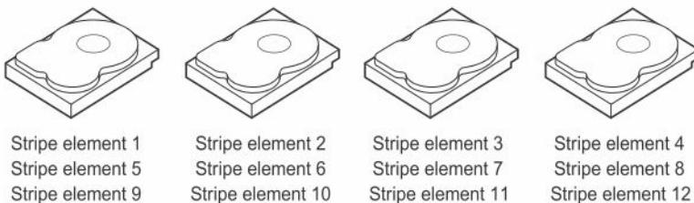
**Figure 6. Example of Disk Striping (RAID 0)**
