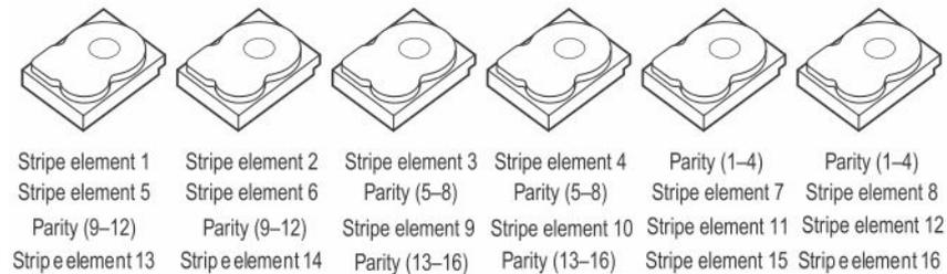
**Figure 9. Example of Dual Distributed Parity (RAID 6)**
