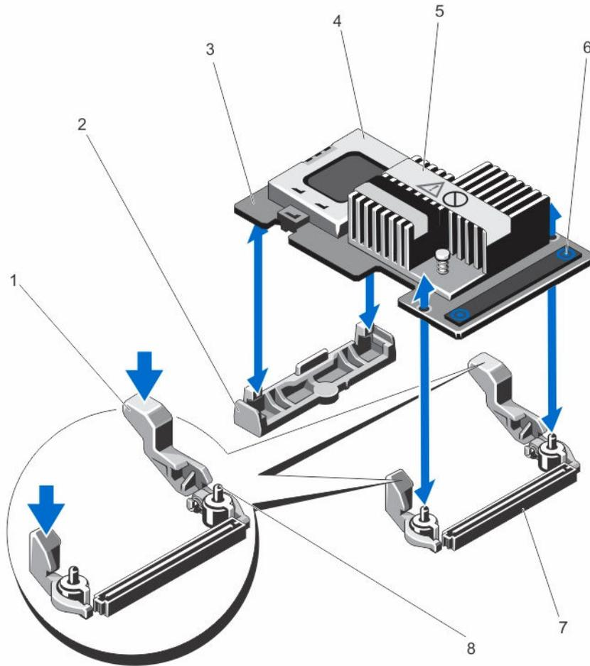
**Figure 3. Removing and Installing the PERC Mini Monolithic Controller**
