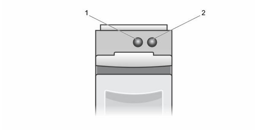
**Figure 5. Disk Carrier LED Indicators**
