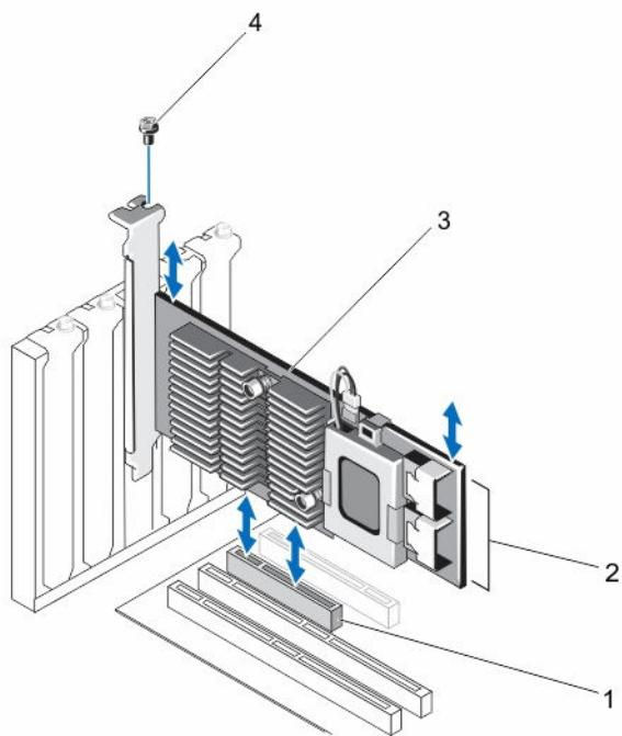
**Figure 1. Removing and Installing the PERC Adapter**
