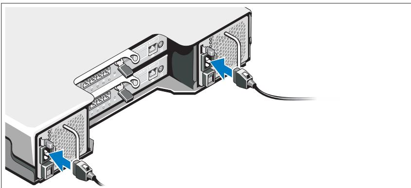
Ensure that the power switch is in the OFF position before connecting the power cables. Connect the system's power cable(s) to the system.
