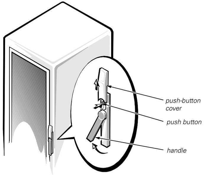
**Figure 3. Opening the 42-U Rack Cabinet Front Door Latch**
