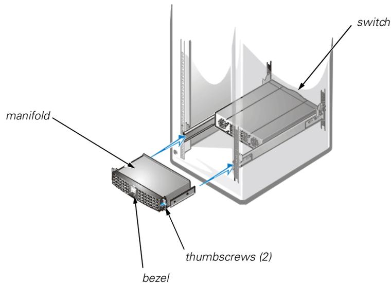
**Figure 9. Installing the Manifold**
