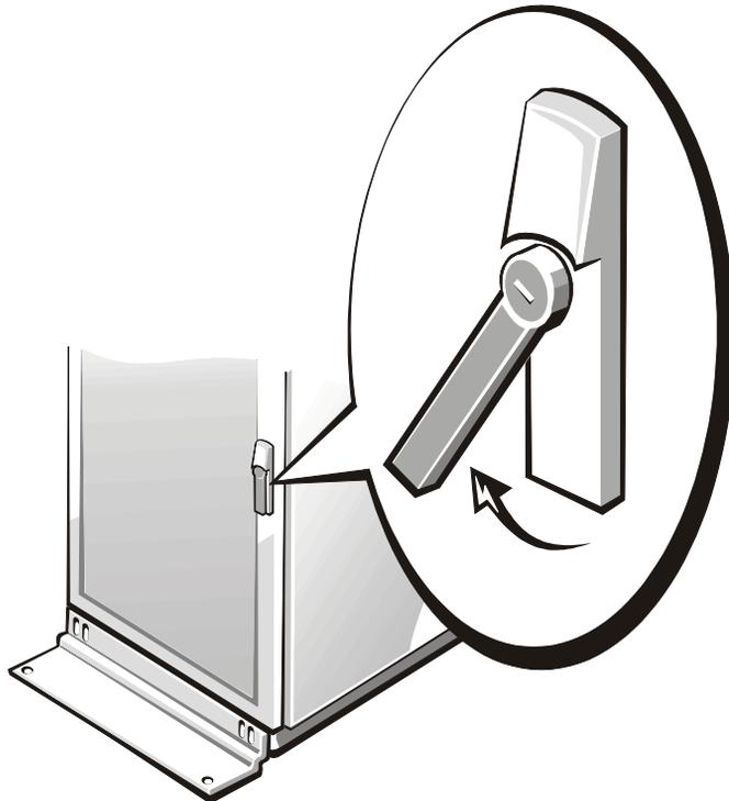
**Figure 2. Opening the 24-U Rack Cabinet Front Door Latch**
