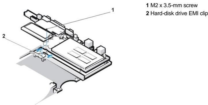
3. Place the system board assembly in the bottom case assembly.
