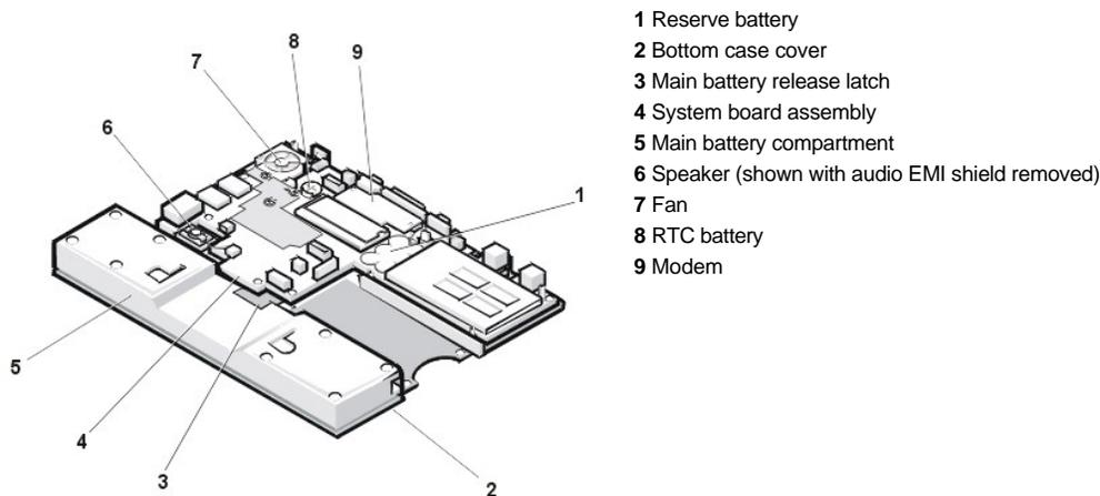
The bottom assembly consists of the following field-replaceable components:
