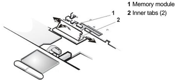
**NOTICE:** To avoid damaging the system board, you must remove the main battery before you service the computer.
