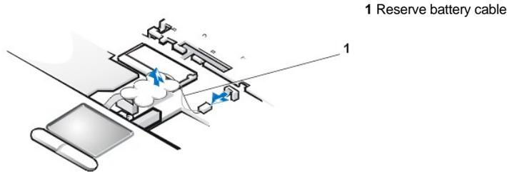
**NOTICE:** The reserve battery provides power to the computer's nonvolatile random-access memory (NVRAM) when the computer is turned off. Removing the battery causes the computer to lose the user-settable parameters in NVRAM. If possible, make a copy of this information before you remove the reserve battery.
