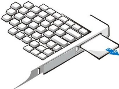
1. Press the PC Card eject button once to pop the button out, and then press the button in again to eject the card partway. (The button may or may not pop out again when you eject the card.)
