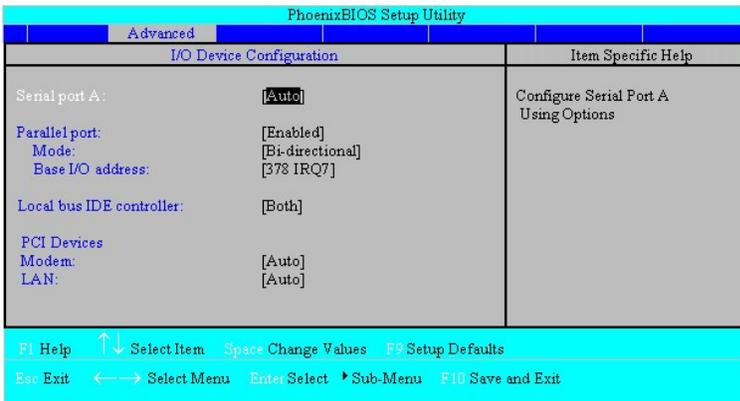
**Table 3. I/O Device Configuration Submenu Options**
