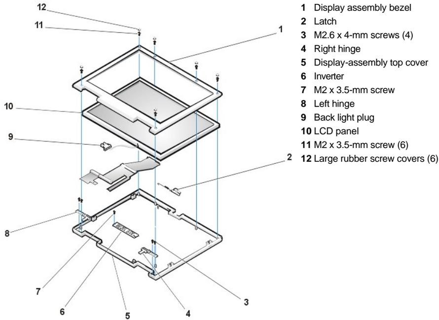
**NOTICE: To avoid damaging the system board, you must remove the main battery before you service the computer.**
