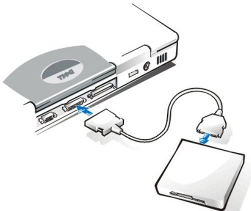
**NOTICE:** When the diskette drive is not being used externally, remove the parallel diskette-drive cable from the parallel connector.
