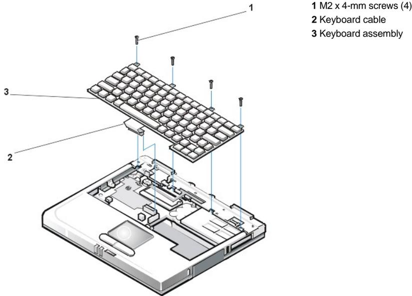
To remove the keyboard assembly, perform the following steps.
