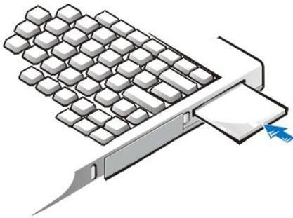
1. If necessary, remove the blank from the PC Card slot. Press the eject button once to pop the button out, press it again to eject the blank partway, and then pull the blank out.
