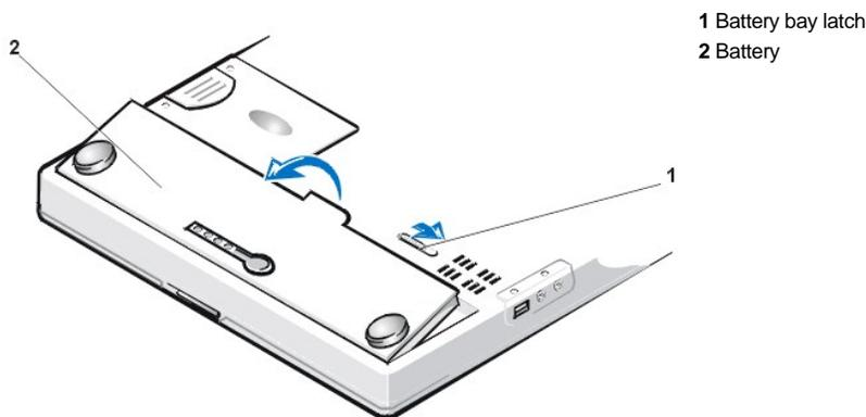
4. Position the new battery as shown in [Figure 2](#), and lower the outside edge of the battery into the battery compartment.
