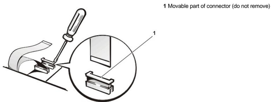
**NOTICE: The ZIF connectors are fragile. To avoid damage, do not apply too much pressure to the movable part of the connector.**
