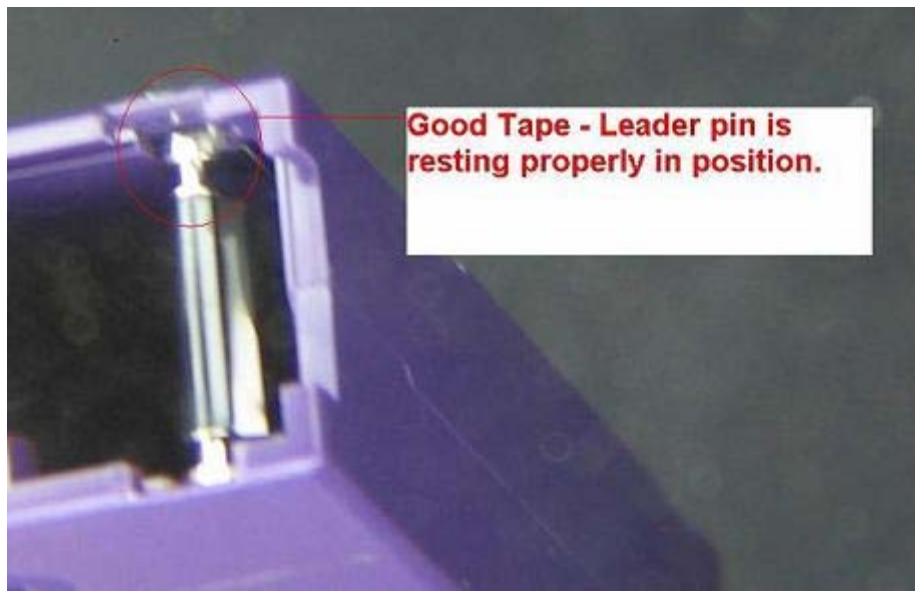
Figure 19- Media Inspection 2- good tape
