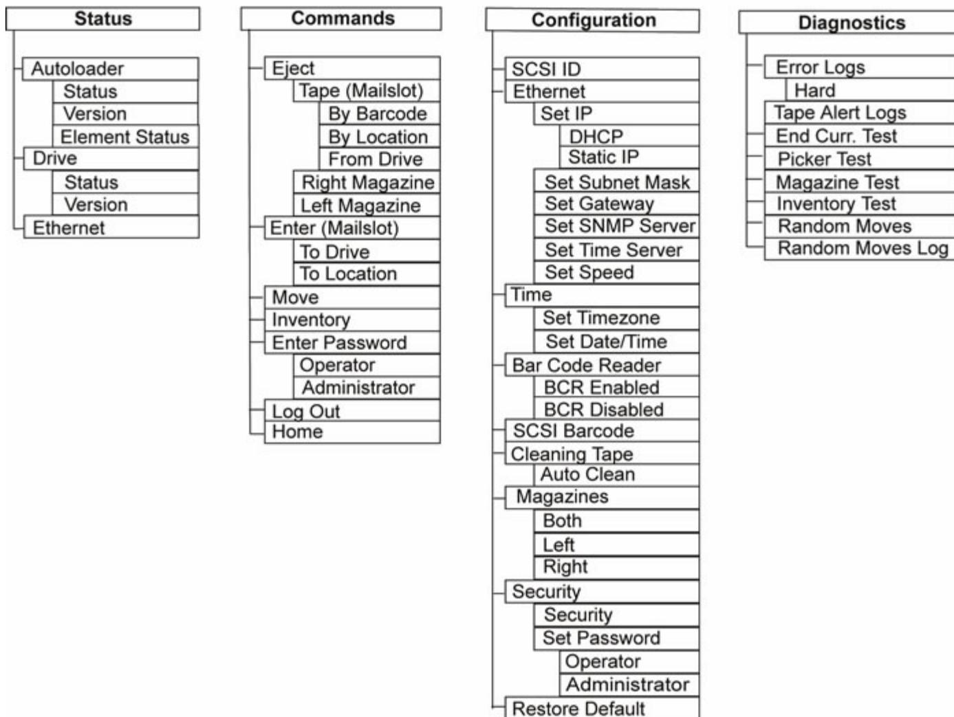
To configure the Dell PowerVault 124T DLT VS160 autoloader, you must verify the setup of the following:
