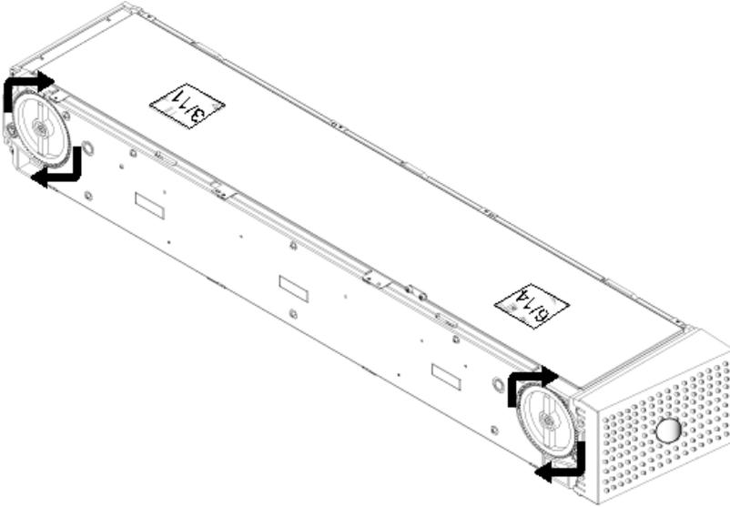
Do not rotate the magazine by inserting your hand and pushing the cartridge carriers. You can use the openings in the magazine to load and unload cartridges from the eight slots within each magazine.
