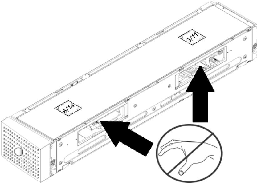
⚠ **Caution:** It is recommended that you fully remove the magazine to load and unload cartridges. If the magazine is not fully removed, do not rotate the magazine.
