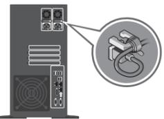
**4** Loop and secure the power cable using the retention strap.
