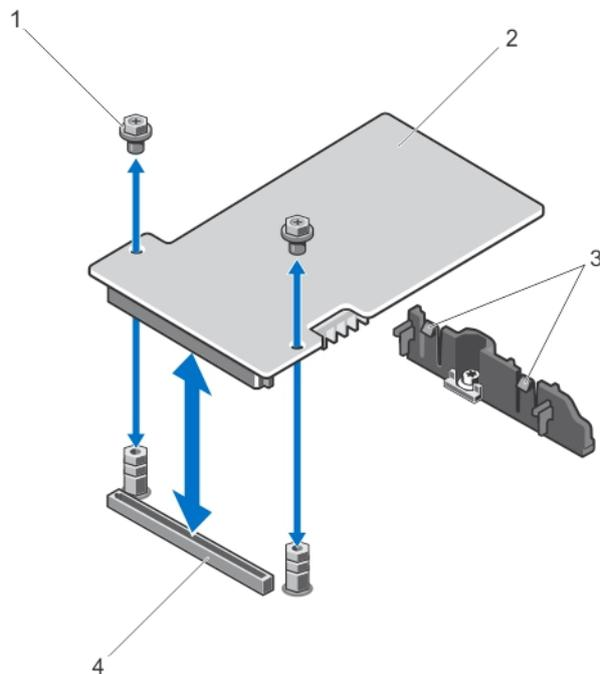
**Figure 25. Removing and installing a storage controller card**
