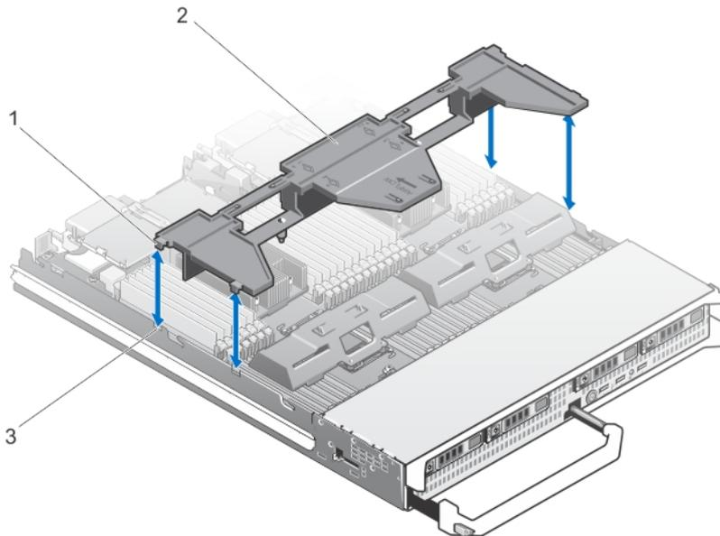
**Figure 7. Removing and installing a cooling shroud**
