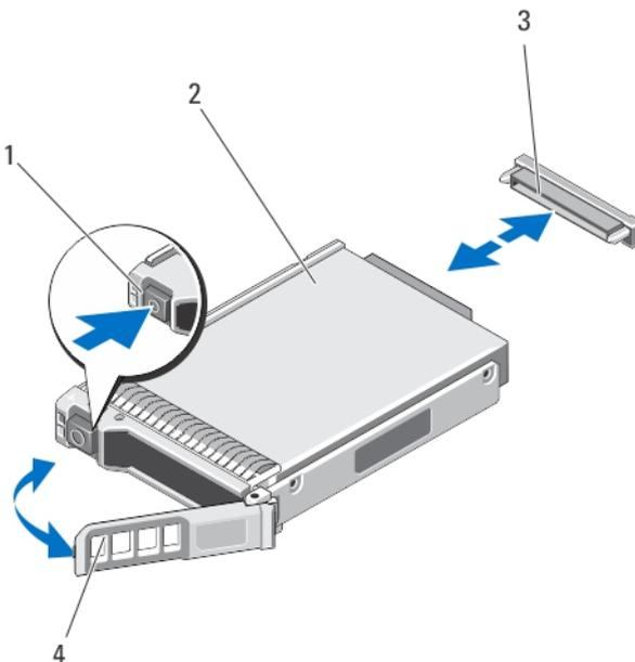
**Figure 8. Removing and installing a hard drive/SSD**
