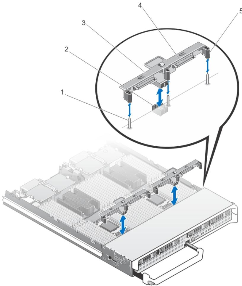
**Figure 11. Removing and installing the hard-drive/SSD backplane (half-length)**
