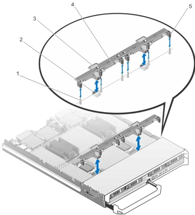
**Figure 10. Removing and installing the hard-drive/SSD backplane (full-length)**
