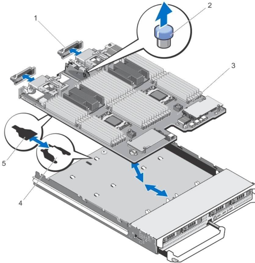
**Figure 21. Removing and installing the system board**
