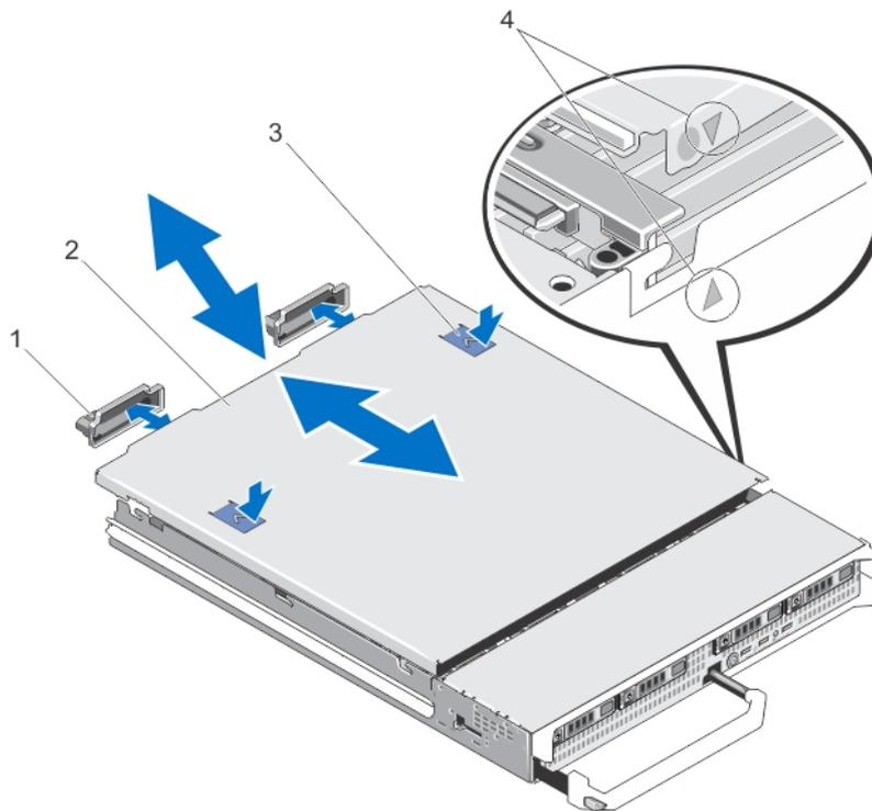
**Figure 5. Opening and closing the server module**
