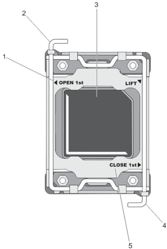
**Figure 19. Processor shield opening and closing lever sequence**
