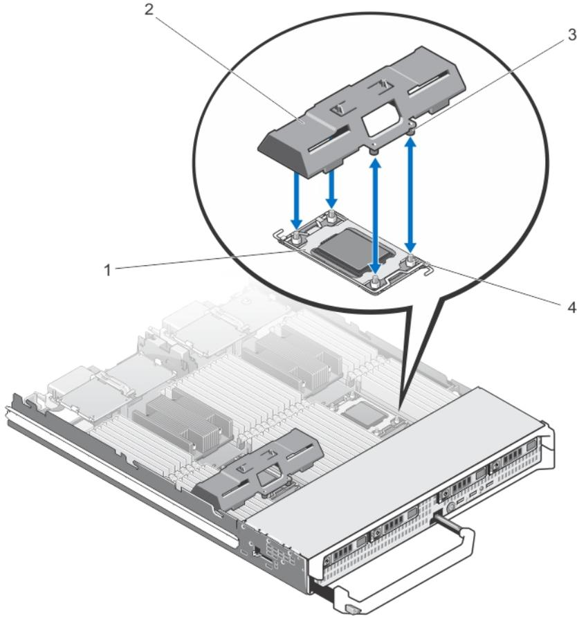
**Figure 17. Removing and installing a processor/DIMM blank**
