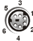
Figure B-4. Pin Numbers for the Keyboard Connector
