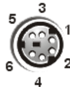
Figure B-5. Pin Numbers for the Mouse Connector
