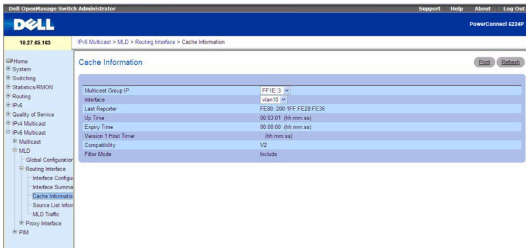
Figure 12-26. MLD Routing Interface Cache Information
