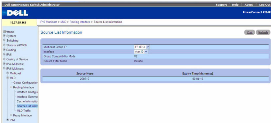
Figure 12-27. MLD Routing Interface Source List Information
