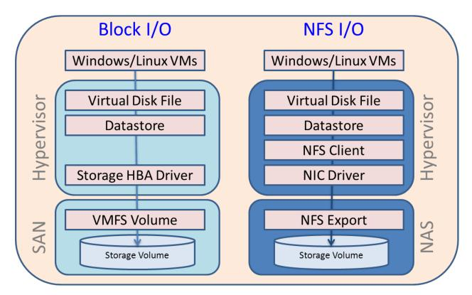
In a SAN, when the VMware hypervisor is using the block-based FC, FCoE, or iSCSI protocol, it creates a VMFS file system on a storage volume (shown as VMFS Volume in Figure 1) to organize and store VMware files. The VMFS file system logic runs on the VMware server.
