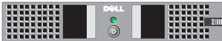
1. On the front of the power module, press and hold the power button for 0.5 seconds.
