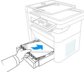
3. Do not exceed the maximum stack height indicated by the paper limit marks on the inside of the tray.
