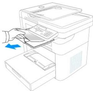
3. If you cannot see the paper in the output tray or the paper does not move when pulled, open the rear cover.
