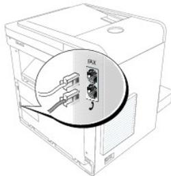
2. To connect a telephone and/or answering machine to your printer, plug the telephone or answering machine into the extension telephone socket ( ).
