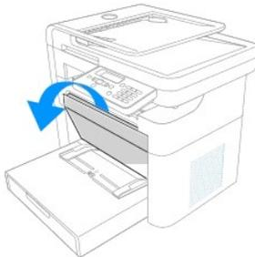
2. Remove the Drum Cartridge by pulling the green handle toward the front of the printer.
