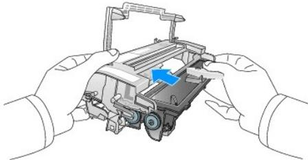
6. Insert the drum cartridge into the printer, using the guiding slots to correctly position the drum. Slide the drum cartridge into the printer until it clicks into place.
