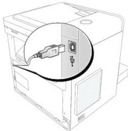
3. Connect the other end of the cable directly into an available USB port on the computer; do not connect the other end to a USB port on a USB keyboard.
