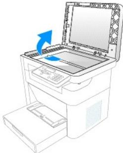
3. Wipe the surface of the scanner glass, underside of the white document cover, and white sheet until they are clean and dry.
