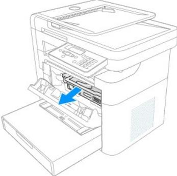
4. The drum cartridge contains the toner cartridge. Set it on a clean flat surface. To prevent damage, do not expose the toner cartridge to light for more than a few minutes.
