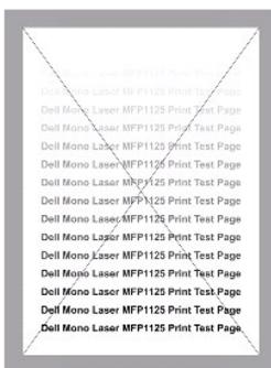
If the test pattern produced appears similar to the images below, the drum may need replacing.
