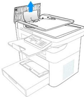
4. Replace the roller and close the ADF cover. Then reload the document into the ADF.
