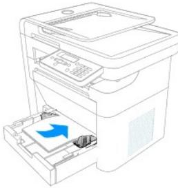
2. Adjust the paper width guide and move it towards the stack of paper until it lightly touches the side of the stack.
