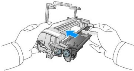
5. Insert the drum cartridge into the printer, using the guiding slots to correctly position the drum. Slide the drum cartridge into the printer until it clicks into place.
