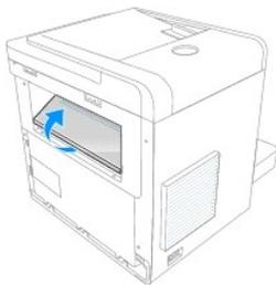
4. Pull the jammed paper out directly upward, to avoid tearing the paper on the rear paper guide parts.
