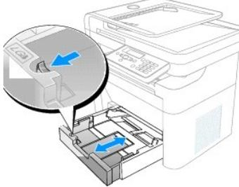
2. Insert the paper stack into the paper tray with the side to be printed on facing down.
