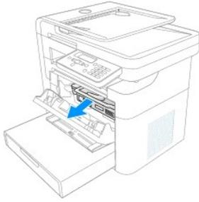
3. Hold the drum cartridge in one hand and push the blue toner release lever in the direction shown to free the toner cartridge.
