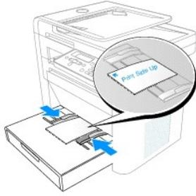
1. Transparencies - load them with the print side up and the top with the adhesive strip entering the printer first
