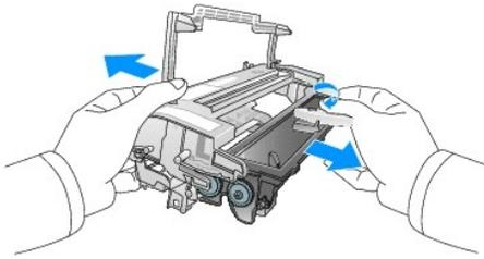
4. Hold the replacement drum cartridge in one hand and push the toner cartridge into the drum cartridge in the direction shown until it clicks into place.
