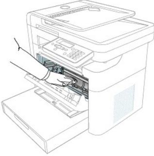
6. Insert the drum cartridge into the printer, using the guiding slots to correctly position the drum. Slide the drum cartridge into the printer until it clicks into place.
