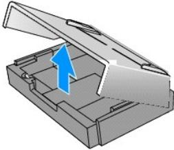
3. Align the tabs on the paper tray with the slots on the printer and push in the direction of the arrow until an audible click is heard.
