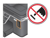
**Warning—Potential Damage:** Do not touch any cables, any network adapter, any connector, the USB Bluetooth adapter, or the printer in the areas shown while actively printing, reading, or writing from a Bluetooth-enabled device. A loss of data can occur.
