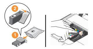
**Note:** Install the new ink cartridges immediately after removing the protective cap to avoid exposing the ink to air.
