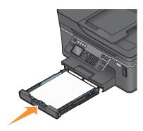
**Note:** If you extended the tray to accommodate A4- or legal-size paper, then the tray sticks out from the front of the printer when inserted.
