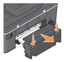
**CAUTION—POTENTIAL INJURY:** The area behind the duplex cover has protruding ribs as part of the paper path. To avoid injury, use caution when accessing this area for clearing a paper jam.
