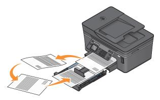
**Note:** To return to single-sided printing, return to the Advanced tab. From the 2-Sided Printing section, select **Off** from the drop-down menu.
