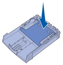
After the tray is inserted, the metal plate springs back up so the paper can feed into the printer.
