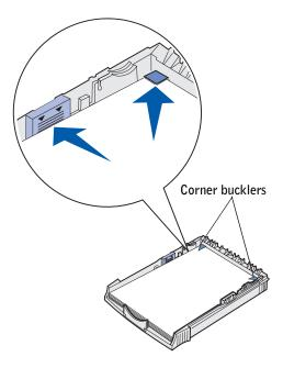
**NOTE:** When you load the tray, do not exceed the maximum stack height indicated by the label in the tray. Overfilling the tray may cause paper jams.
