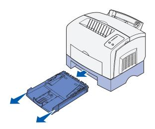
**2** Make sure the metal plate is pressed down before inserting the tray into the printer.
