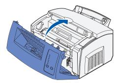
If you cannot close the printer cover, make sure the toner cartridge is positioned correctly. Do not force the cover closed.
