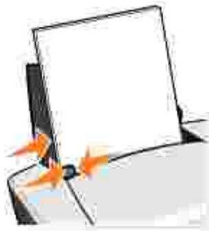
**NOTE:** Load letterhead paper with the top of the letterhead entering the printer first and facing up.
