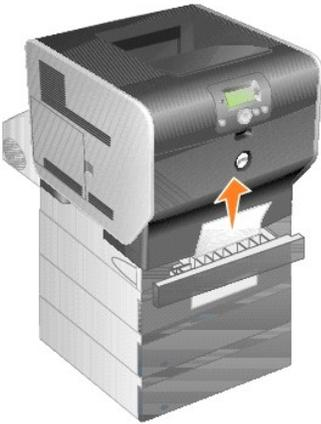
3. Open any optional trays beginning at the top, and remove any jammed media.
