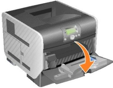
2. Push the release latch to the right to open the top front cover.
