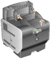
6. Rotate the tray up until the upper tabs *snap* into the upper slots.
