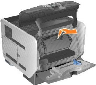
5. Locate the used transfer roller on the bottom of the inside of printer.
