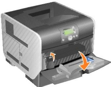
3. Align the tabs on the envelope feeder with the slots on both sides of the printer, and then gently push the envelope feeder into the opening until it *snaps* into place.
