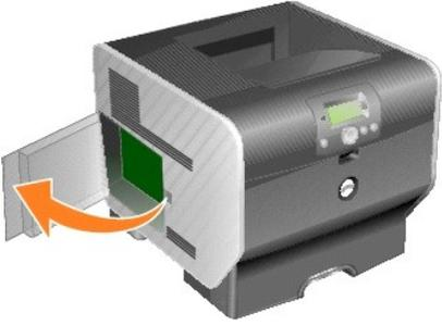
**NOTE:** If an option card has been installed, you may need to remove the option card before installing the Font ROM.
