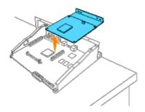
7. Insert the controller card into the printer.
