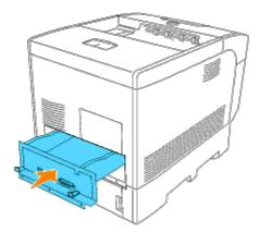
7. Tighten the three screws on the controller card from the back side of the printer.
