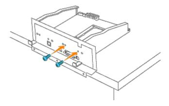
7. Insert the controller card into the printer.
