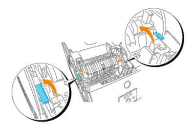
4. Grip the knobs and gently lift the fuser out of the printer.
