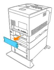
9. Pull the printer's tray out until it stops. Hold the tray with both hands, lift the front slightly and remove it from the printer.
