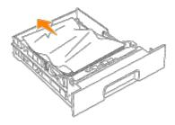
3. Pull the jammed paper out carefully to avoid tearing it. If the paper is torn, confirm that there are no scraps of paper remaining inside the printer.
