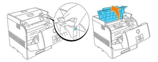
3. Grab the imaging drum by the handle, and pull it up and out.
