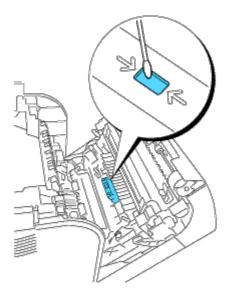
**NOTE:** Do not allow anything hard to come in contact with the automatic density control (CTD) sensor window. Do not use excessive force to clean the window.
