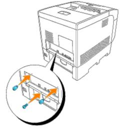
9. Reattach the paper tray cover to the back of the printer.
