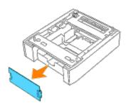
4. Gently pull out the tray of the optional 500-sheet tray module until it stops. Hold the tray with both hands, lift up the front slightly and remove it from the tray module.
