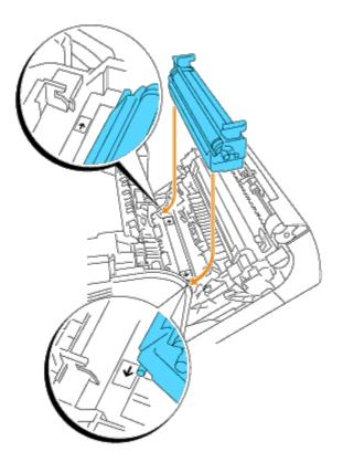
7. To lock the transfer roller into the printer push down the tabs until you hear a click.
