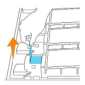
**NOTE:** Pull the toner seal straight up. Pulling the toner seal diagonally may tear the seal.
