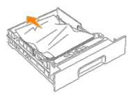
10. If there is jammed paper remaining inside the printer, pull it out carefully to avoid tearing it.
