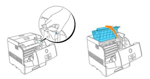
3. Remove the protective cover from the imaging drum.
