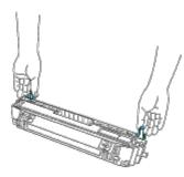
2. Align the arrow marks on the transfer roller to the marks on the printer, and gently push the roller into the printer.
