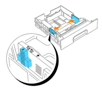
3. Squeeze the length guide and slide it to the edge of the tray.
