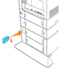
hook as shown in the graphic, and lightly pull the power cable. Then, plug the other end of the cable into the grounded outlet.
