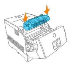
2. Completely push down the fuser by holding the knobs at both ends of the fuser until the levers next to both ends of the fuser return to their original position.
