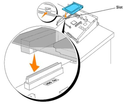
6. Align the two protrusions with the holes on the controller card, and then tighten the two screws from the back side of the controller card.
