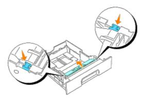
3. Gently raise the separator roller assembly, and slide it to the left.
