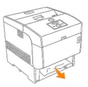
11. If jammed paper cannot be found, pull down the blue cover along the top of the hole where the tray cartridge was in the printer, and pull the jammed paper out carefully. Close blue cover after removing jammed paper.
