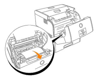
**NOTE:** If a paper jam occurs in the fuser area, a sheet of paper may already have been fed from the tray. Make sure there is no paper remaining inside the printer, using step 8 through 14.
