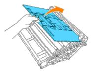
CAUTION: Make sure nothing touches or scratches the surface of the light-sensitive drum surface (green-colored roller) or the transfer roller (black-colored roller). Scratches, dirt, or oil from your hands on the imaging drum or transfer roller may reduce the print quality.
