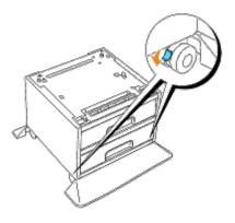
CAUTION: Failure to lock down the brakes can cause the printer to move unexpectedly, resulting in injury.
