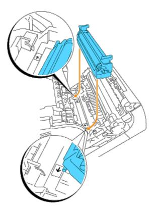
5. To lock the transfer roller into the printer push down the tabs until you hear a click.
