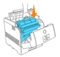
6. Pull the protective cover on the imaging drum straight up to remove it.
