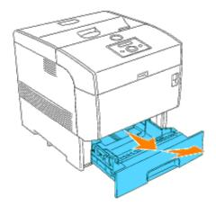
2. Slide the width guides to the edge of the tray. The width guides should be fully extended.
