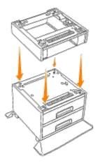
6. Insert the four screws provided into the four holes inside the optional 500-sheet tray module and tighten them with a coin to secure the 500-sheet tray module to the optional 1000-sheet tray module.
