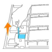
**NOTICE:** Pull the toner seal straight up. Pulling the toner seal diagonally may tear the seal.
