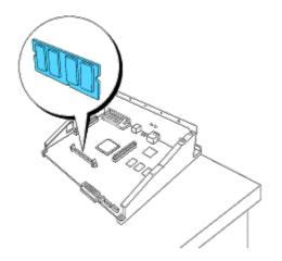
6. Push the memory card into the slot firmly.
