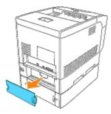
4. Pull the printer's tray out until it stops. Hold the tray with both hands, lift the front slightly and remove it from the printer
