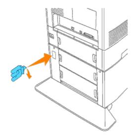
10. Plug the power cable into the power cable connecter at the back of the printer, wind the power cable onto the cable hook as shown in the graphic, and lightly pull the power cable. Then, plug the other end of the cable into the grounded outlet.
