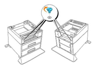
7. Lift the printer and align the four guide pins of the optional 500-sheet tray module with the holes at the bottom of the printer.
