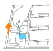
**NOTICE:** Pull the toner seal straight up. Pulling the toner seal diagonally may tear the seal.
