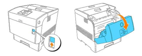
2. Push the button as shown in the following illustration and open the imaging drum cover.
