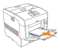
4. Slide the width guides until they rest lightly against the edge of the print media stack.
