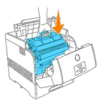
3. Pull the protective cover on the imaging drum straight up to remove it.
