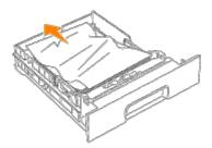
3. If there is jammed paper remaining inside the printer, pull it out carefully to avoid tearing it.
