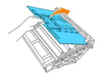
4. Holding the imaging drum by the handle with the flat part facing the back of the printer, align the plastic guides on both sides of the imaging drum with the slots in front of the arrows on the printer. Gently lower the imaging drum into the printer.
