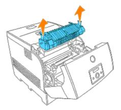
5. Unpack a new fuser, grip the fuser by the knobs, align it with the slots in the printer, and slowly push it in.
