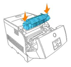
6. Completely push down the fuser by holding the knobs at both ends of the fuser until the levers next to both ends of the fuser return to their original position.
