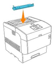
7. Grip the levers at each end of the toner cartridge with your fingers, then push down firmly to rotate the levers forward.
