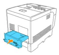
8. Tighten the three screws on the controller card from the back side of the printer. The two screws on the upper side are different in shape from the one on the lower side. Be careful not to confuse them.
