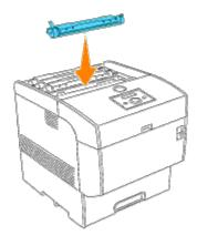
4. Grip the levers at each end of the toner cartridge with your fingers, then push down firmly to rotate the levers forward.
