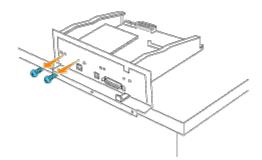
6. Hold the multi protocol card and remove it from the controller card.
