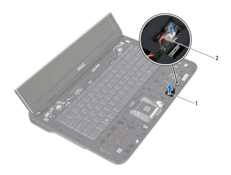
1 coin-cell battery 2 coin-cell battery cable
