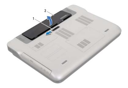
battery release latch battery
