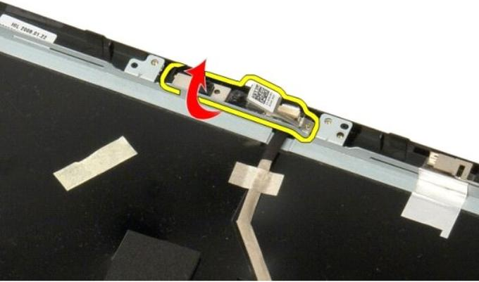
6. Release the display camera data cable from its clip and disconnect the display camera data cable.
