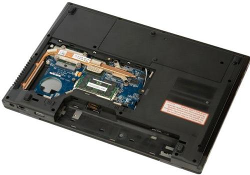
4. Remove the screw that secures the optical drive in place.
