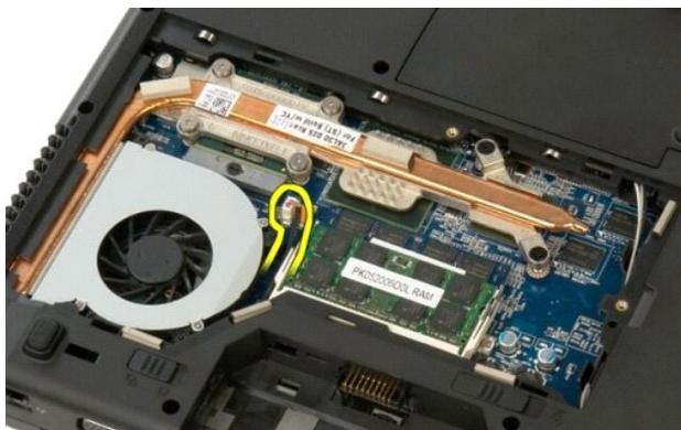
5. Remove the three screws that secure the fan to the computer.
