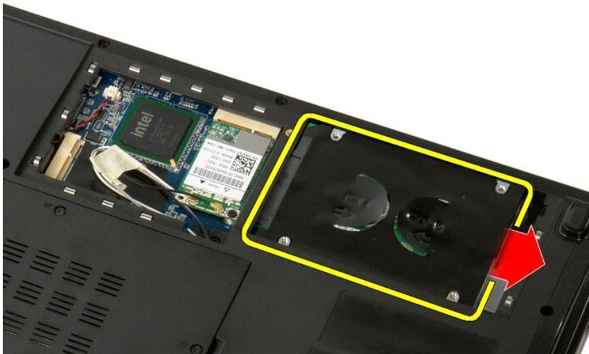
5. Lift and remove the hard drive from the computer.
