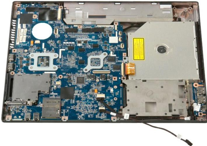
12. Remove the screw that secures the USB/1394 connector board to the computer chassis.
