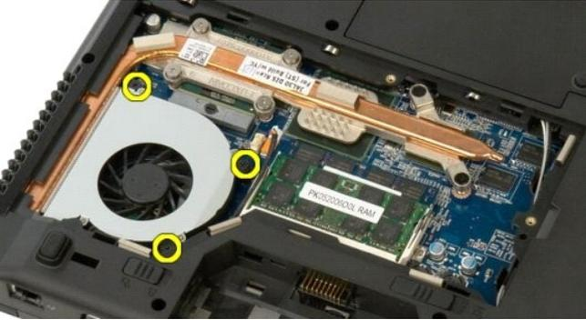
6. Lift the fan and remove it from the computer.
