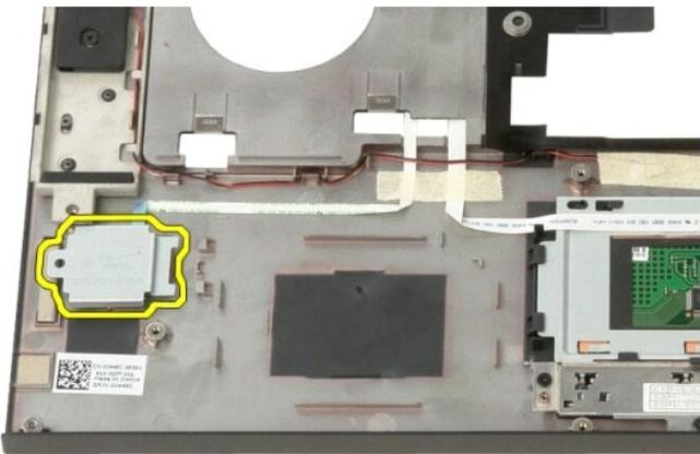
13. Open the fingerprint cable retention clip.
