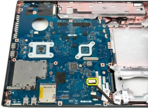
19. Disconnect the second data cable from the system board.
