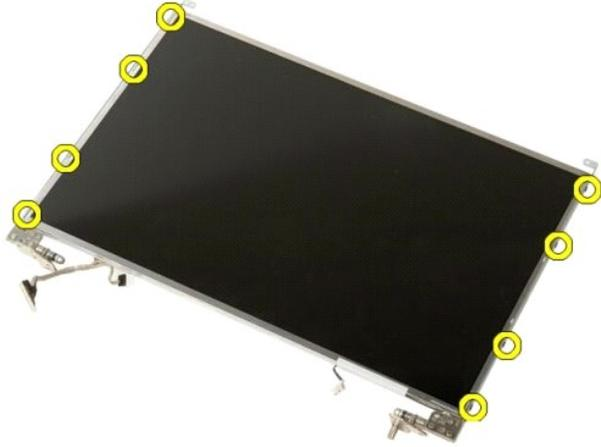
7. Slide the hinges away from the display panel assembly.
