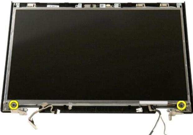
5. Remove the LCD display panel from the display assembly.
