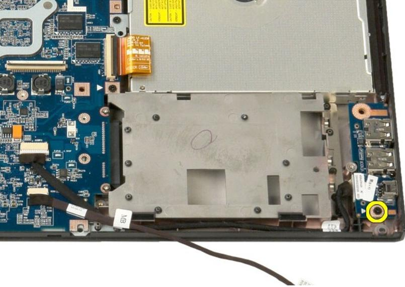
13. Lift the USB/1394 connector board from its slot.
