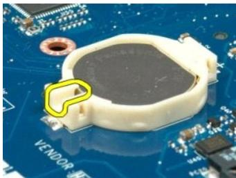
20. Remove the coin-cell battery.
