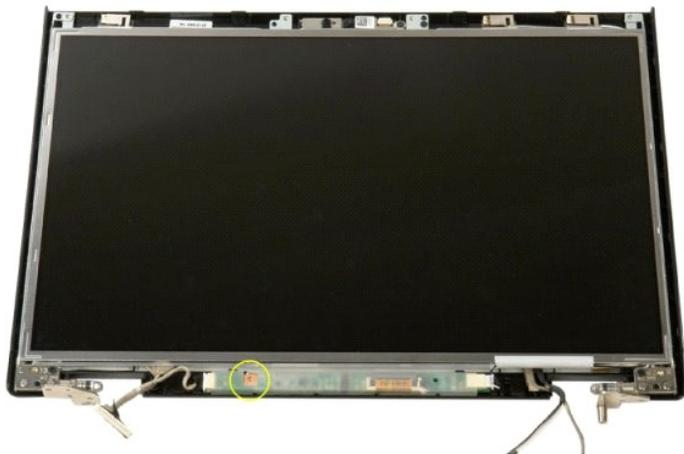
4. Open the display inverter data cable clip.
