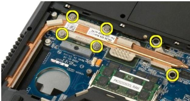
6. Lift the edge of the heat sink that is closest to the center of the computer.
