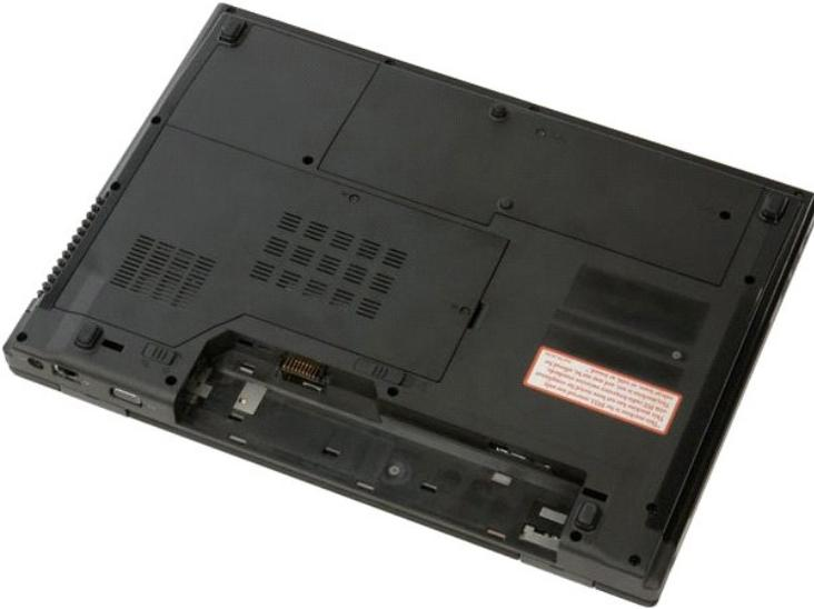
3. Remove the two screws that secure the hard drive and mini-card access panel to the computer.
