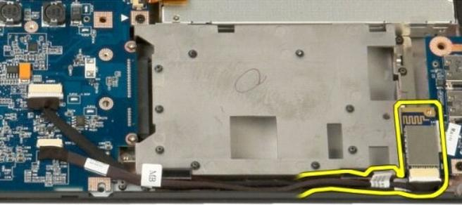
12. Disconnect the data cable from the Bluetooth module.
