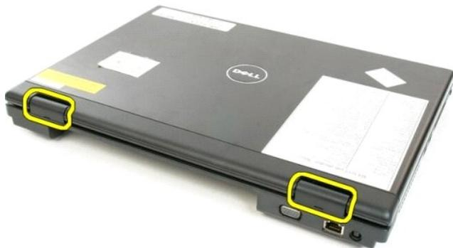
4. Starting on the right side, separate the hinge cover from the base of the computer.
