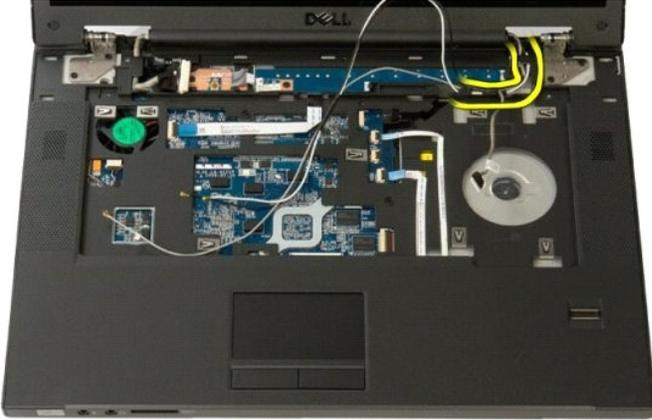
13. Remove the display data cable from its routing slot.
