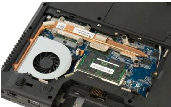
4. Disconnect the fan cable from the system board.
