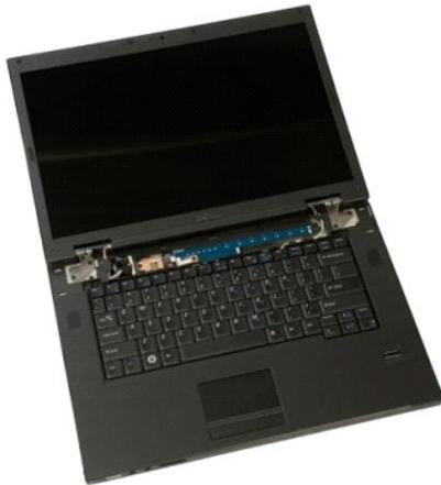
4. Remove the two screws that secure the keyboard to the computer.
