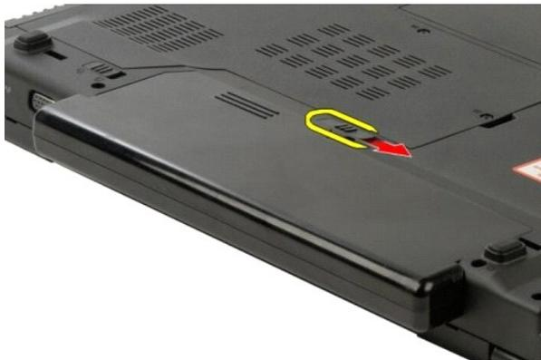
4. Slide the battery itself toward the back of the computer and remove.
