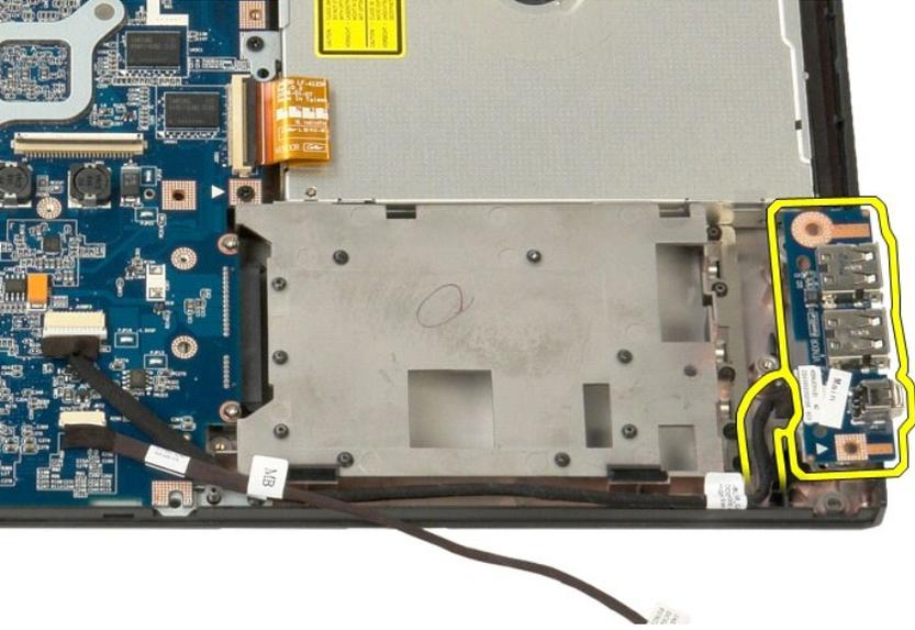
15. Lift the inside edge of the USB board and remove the board from the computer.
