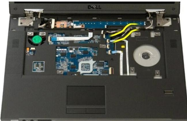
12. Remove the antenna cables from their routing slots.
