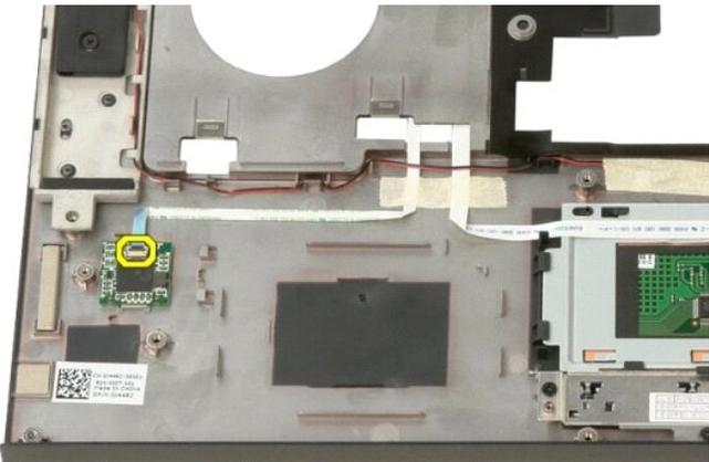
14. Remove the fingerprint cable from the retention clip.
