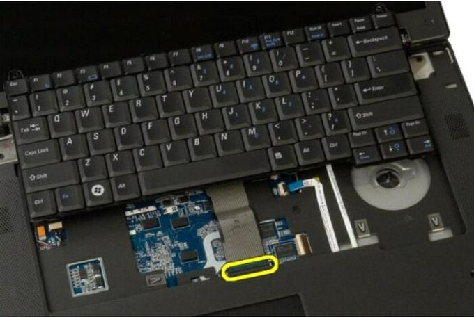
7. Remove the keyboard data cable from the clip.
