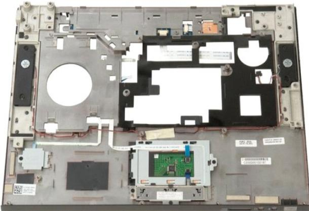
12. Remove the four screws that secure the speaker assembly to the palm rest.
