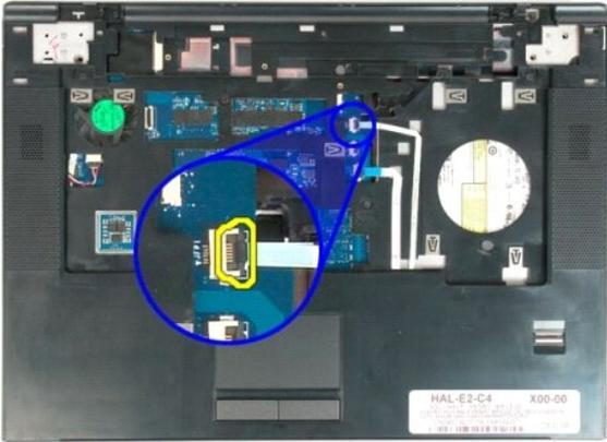
11. Remove the fingerprint reader data cable from the clip.
