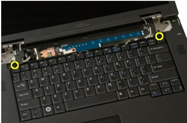
5. Lift the back edge of the keyboard slightly and slide the keyboard toward the back of the computer.
