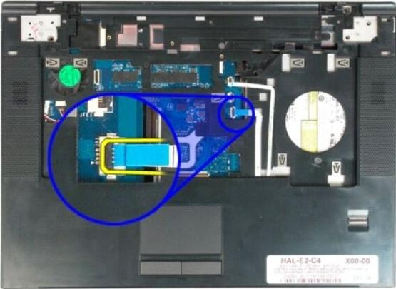
14. Remove the four screws that secure the palm rest to the top of the computer.
