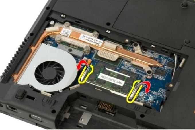
5. Remove the memory module from the socket.
