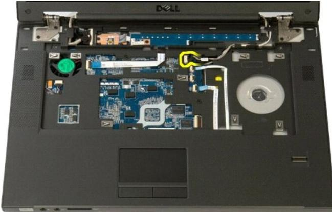
10. Disconnect the display data cable from the system board.
