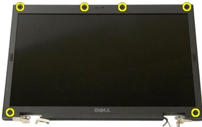
4. Remove the six screws that secure the bezel to the display assembly.
