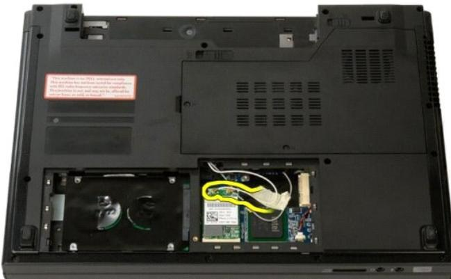
9. Disconnect the camera cable from the system board.
