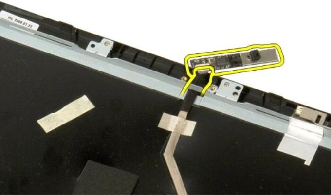
7. Remove the display camera from the display assembly.
