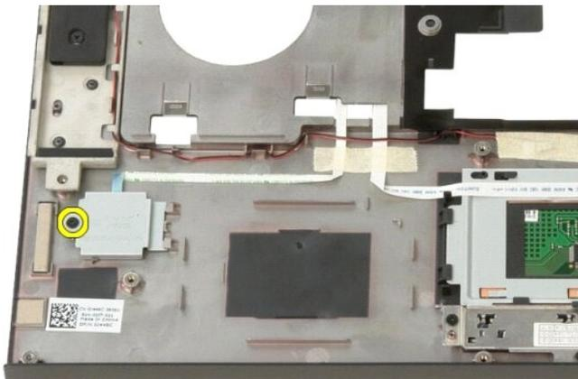
11. Slide the fingerprint reader retention plate to the left.
