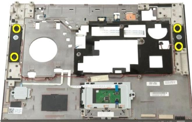
13. Lift the speakers from their slots, then remove the speaker assembly from the computer.
