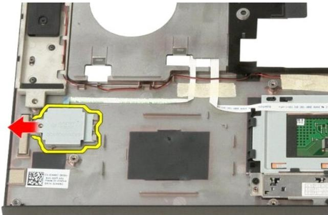
12. Remove the fingerprint reader retention plate.
