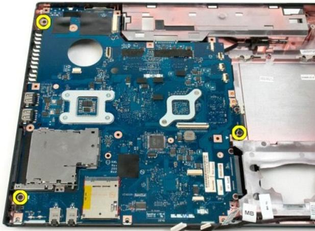
21. Remove the system board from the computer chassis.
