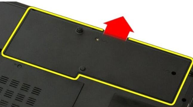
5. Remove the hard drive and mini-card access panel.
