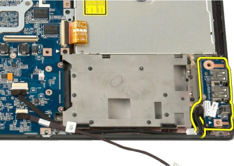
14. Disconnect the data cable from the USB/1394 connector board.
