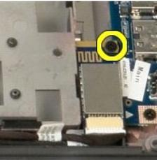
11. Lift the edge of the Bluetooth module closest to the front of the computer and lift the module from its slot.
