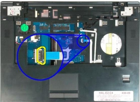
13. Remove the touch pad data cable from the clip.
