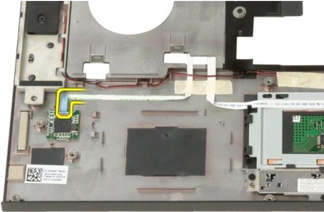
15. Remove the fingerprint reader from the palm rest.
