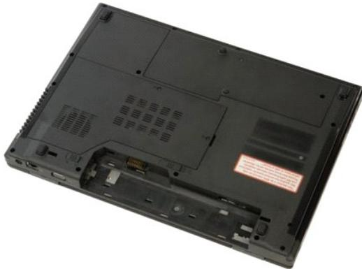
3. Loosen the two captive screws on the access panel.
