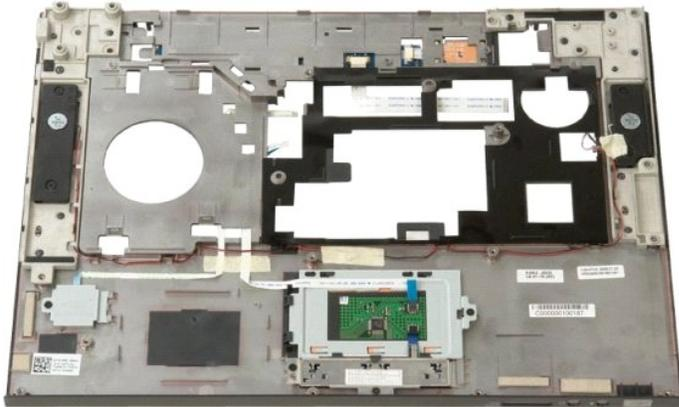
10. Remove the screw that secures the fingerprint reader retention plate to the computer chassis.
