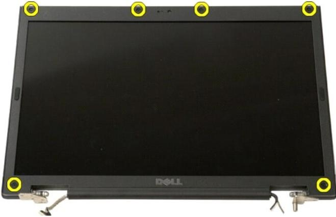
5. Remove the bezel from the display assembly.
