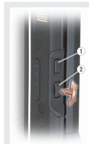
1 **Back button** — Use the back button to move backward in applications that support navigation, such as web browsers and Windows Explorer, and to close the active window. To move backward, press and release the back button. To close the active window, press and hold the back button.
