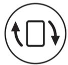
3 **Screen rotate button** — Use the screen rotate button to change the display orientation from portrait to landscape mode; each time you press and release the screen rotate button, the screen image rotates clockwise 90 degrees. To switch off the screen, press and hold the screen rotate button; press and hold the button a second time, or use the pen to wake the Tablet-PC.
