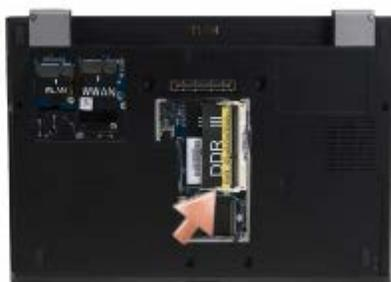
5. Push the long edge of the memory module down until the retaining clips lock the module into place.
