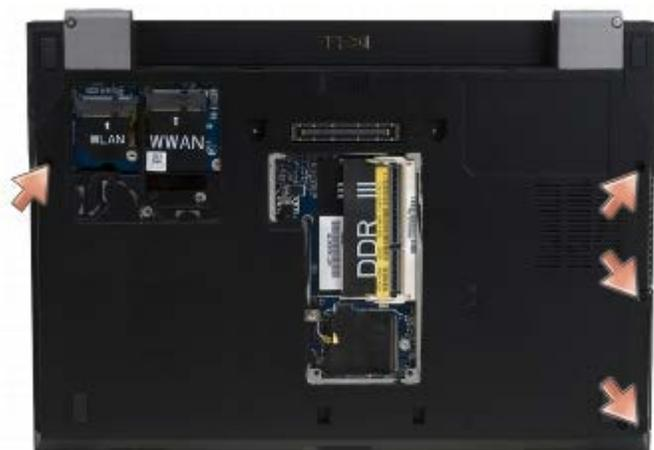
6. Turn the computer rightside-up and remove the five M2.5 x 5-mm screws and five M2.5 x 8-mm screws from the top of the palm rest.
