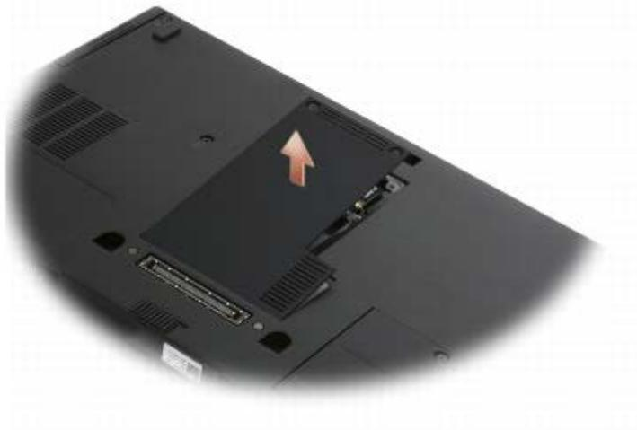
**NOTICE:** To prevent damage to the memory module connector, do not use tools to remove or replace the memory module.
