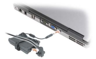
The AC adapter converts AC power to the DC power required by the computer. You can connect the AC adapter with your computer turned either on or off.
