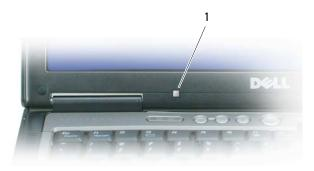
1 ambient light sensor The ALS is disabled when your computer is shipped to you. If you enable the ALS and then use any of the display brightness key combinations, the ALS is disabled and the display brightness is increased or decreased accordingly.
