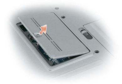
**MEMORY MODULE COVER** — Covers the compartment that contains the second memory module connector (DIMM B) (see "Memory" on page 146).
