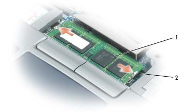
1 memory module (DIMM A) 2 securing clips (2)
