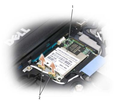
1 WLAN card 2 antenna cables (2)
