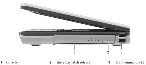
**DRIVE BAY** — Supports a floppy or an optical drive, second battery, second hard drive, or a Dell TravelLite<sup>™</sup> module (see "Using Multimedia" on page 59).
