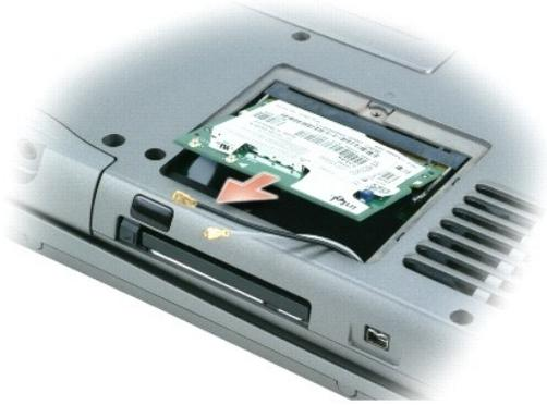
➔ **NOTICE:** In the next step, ensure that the antenna cables extend over the edge of the computer, so that they are not trapped beneath the new Mini PCI card.
