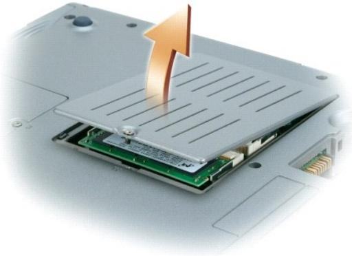
**➡ NOTICE:** To prevent damage to the memory module connector, do not use tools to spread the securing clips that secure the memory module.
