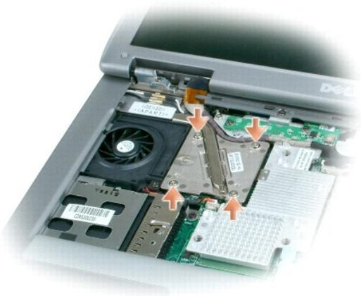
9. Lift the microprocessor thermal-cooling assembly up and to the right to remove it from the system board.
