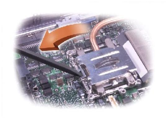
4. Close the microprocessor retaining clip.
