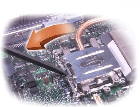
4. Close the microprocessor retaining clip.
